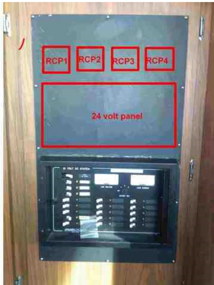
Figure 17.4-22: Proposed 24V Power distribution and RPC location
