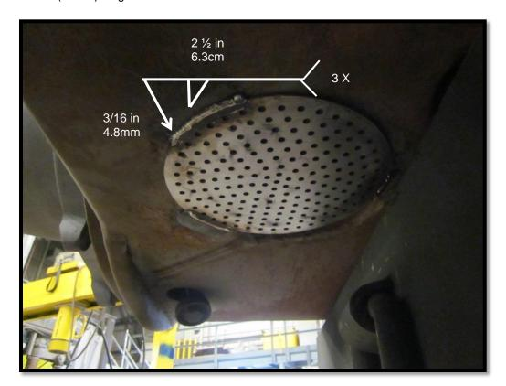
2.1.3.4. Install the 5 in plate (12.7 cm) # 108129547 in the crew compartment by the escape hatch.
