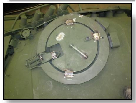
2.3. For the Drivers hatch, close the hatch and weld the hatch locking mechanism in place.
