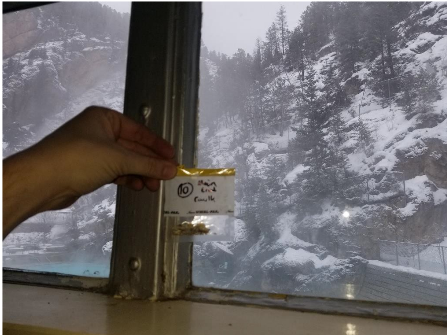
Photograph 10: Silver Lead-Based Paint on South Window Frames
