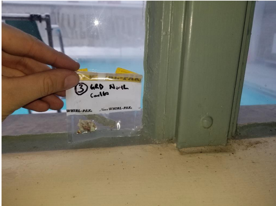
Photograph 8: Green Lead-Based Paint on Window Frames
