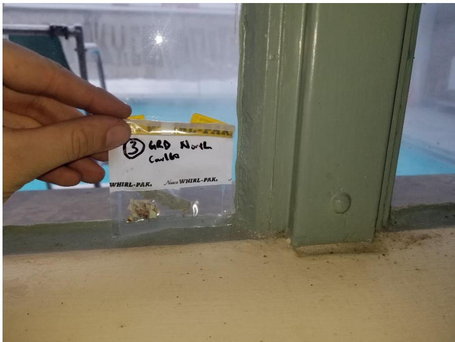
Photograph 2: Asbestos-Containing Window Caulking Ground Floor North
