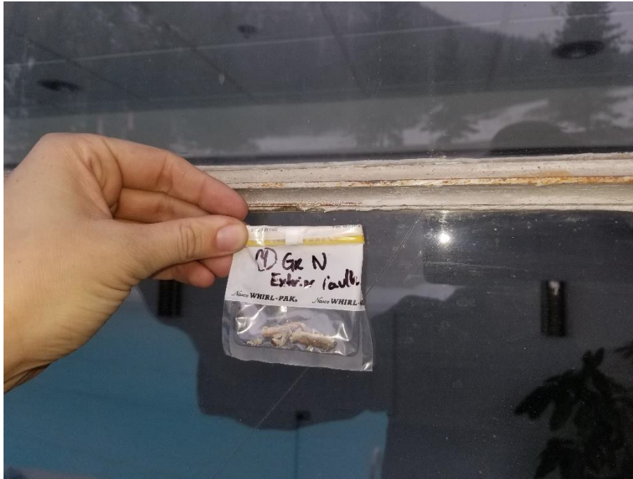
Photograph 3: Asbestos-Containing Window Caulking Ground Floor North
