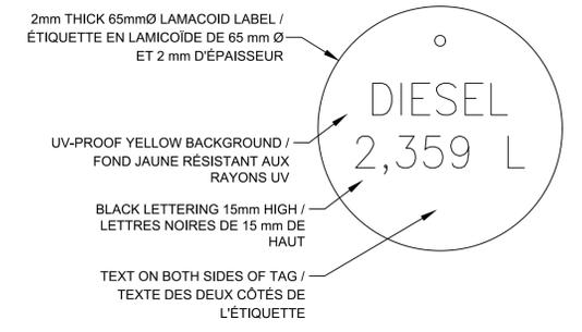
**9 TAG AT FILL CONNECTION / ÉTIQUETTE AU NIVEAU DU RACCORD DE REMPLISSAGE**
