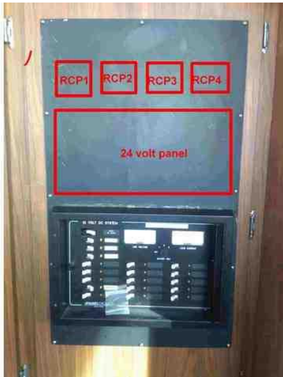
Figure 17.4-22: Proposed 24V Power distribution and RPC location
