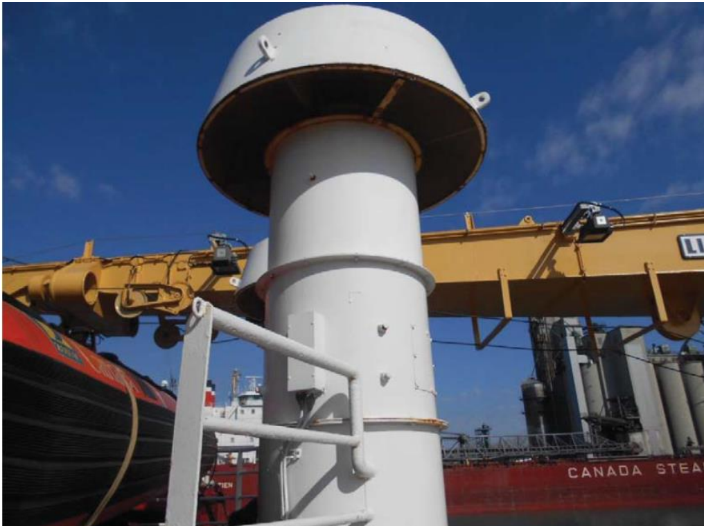
Figure 16.3-3: Photograph of in-situ engine room Supply Fan (SF-5 or SF-6)
