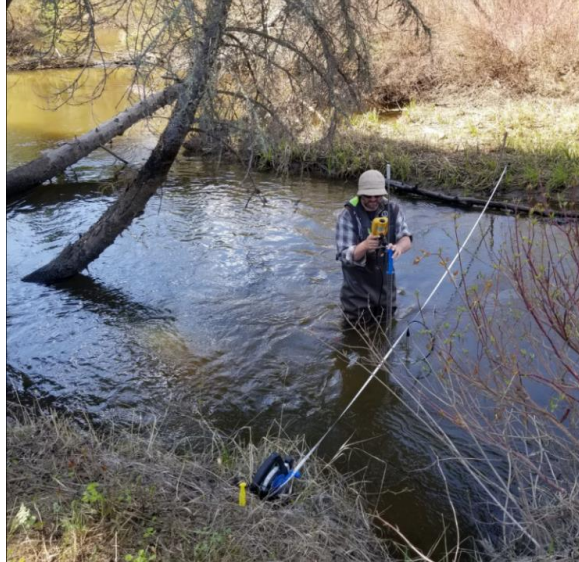
Figure 2: A technologist performing a hydrometric measurement at 07DA040 Big Creek near the Mouth
