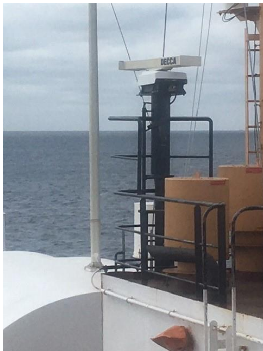
Pictures: Aft Looking Radar (Display C) and Associated Equipment
