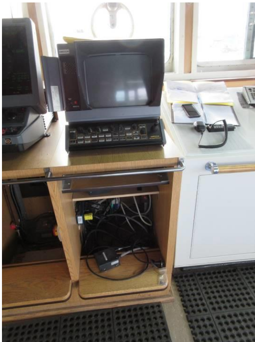
Pictures: Aft Looking Radar (Display C) and Associated Equipment
