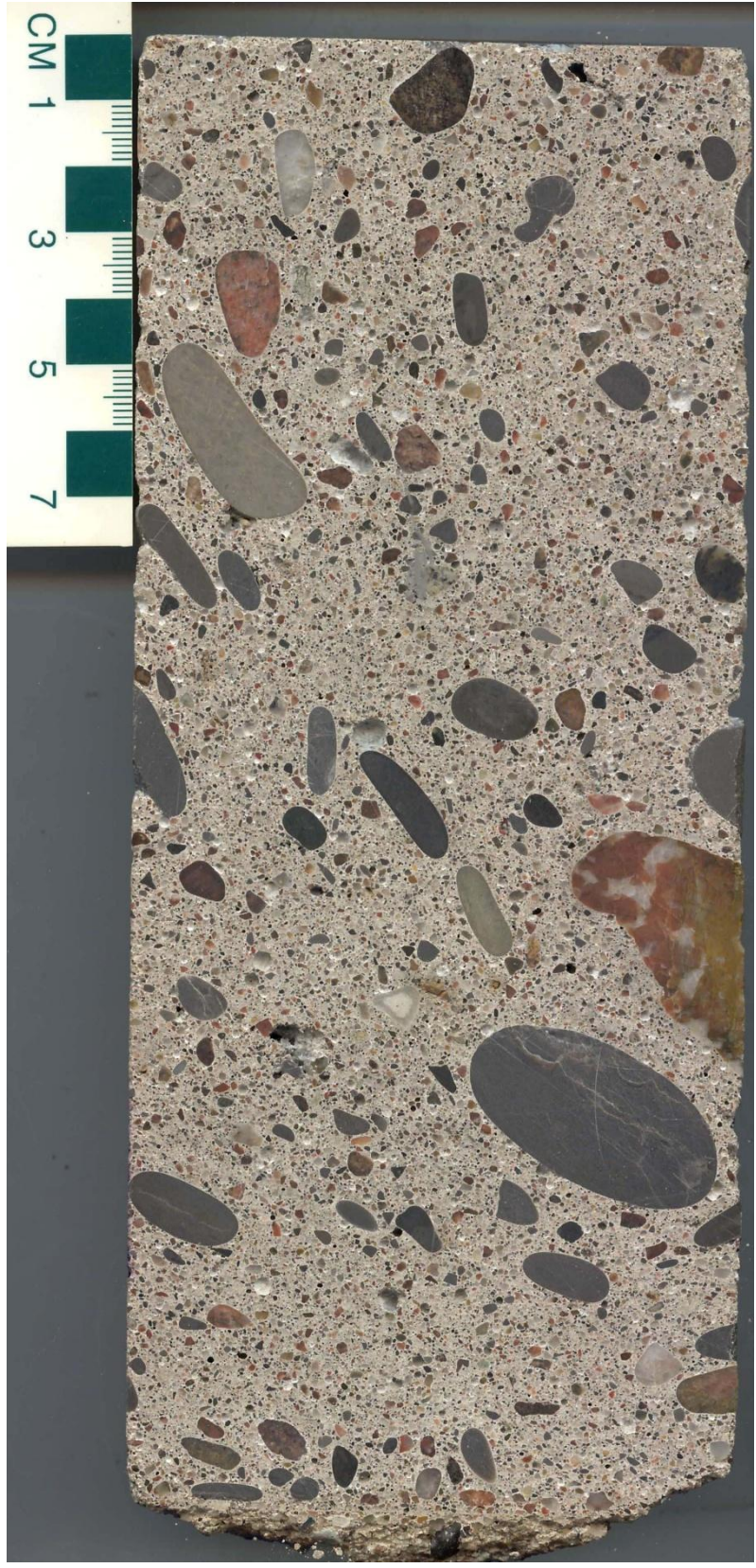
Figure 1: Core 1. Note preferred orientation of long axis of coarse aggregate particles.
