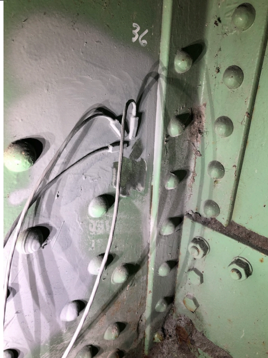
Figure13: Test Location 36 at South Trunnion Exterior Plate Location (Readings Taken on Interior Surface of Plate)
