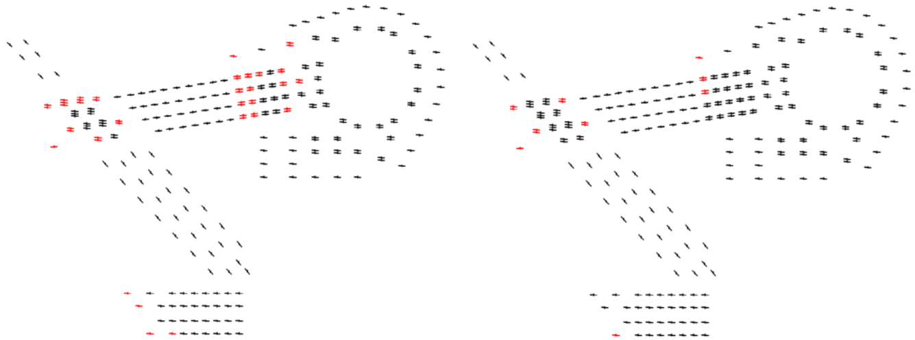
Figure 24 - Fasteners with insufficient shear resistance at undeteriorated state for upper bound fastener stiffness (a) Left: ULS B1 to ULS B3 (b) Right: ULS 1
