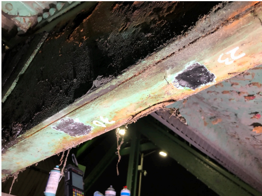
Figure10: Test Locations 23 and 30 at South Trunnion Plate Interior Location (Readings Taken from Inside Bottom Surface of Angle)
