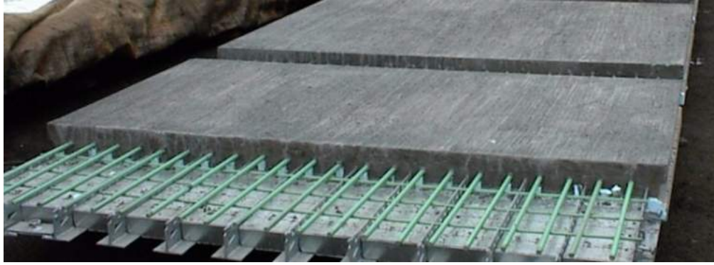
Figure 4: Exodermic deck cross section (photo credit http://www.faddis.com/product/bridge-decks/ )
