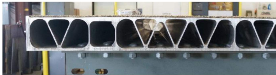
Figure 6: Florida DOT Aluminum Orthotropic Deck Test Panel, with wearing surface, bolted on steel stringer 10
