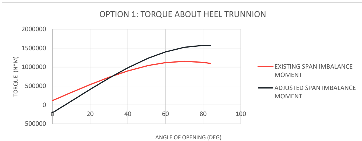
Figure 9: Option 1: Torque about Hell Trunnion
