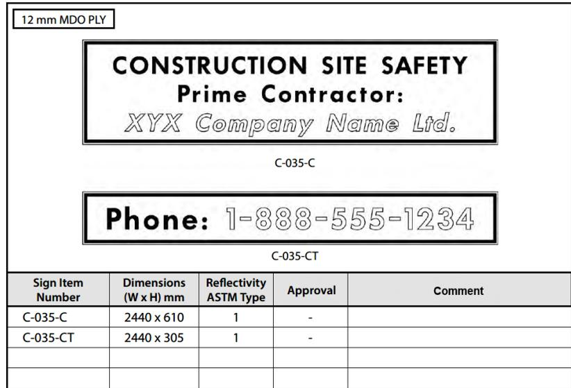
Figure 01 35 00 – 03: Sign C-035-C and C-035-CT Details
