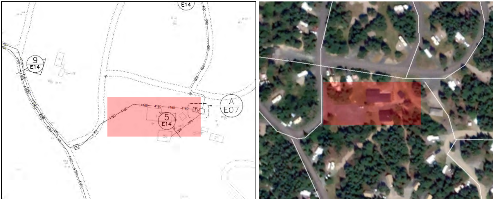
Figure 4: Newman Sound Campground Underground Electrical Primary Recapitalization. Left: Area in Sheet E07 showing the installation of new underground cable outside existing roadway. Right: Google Earth image of same area showing the approximate location of project activity area (Crandall 2019c).
