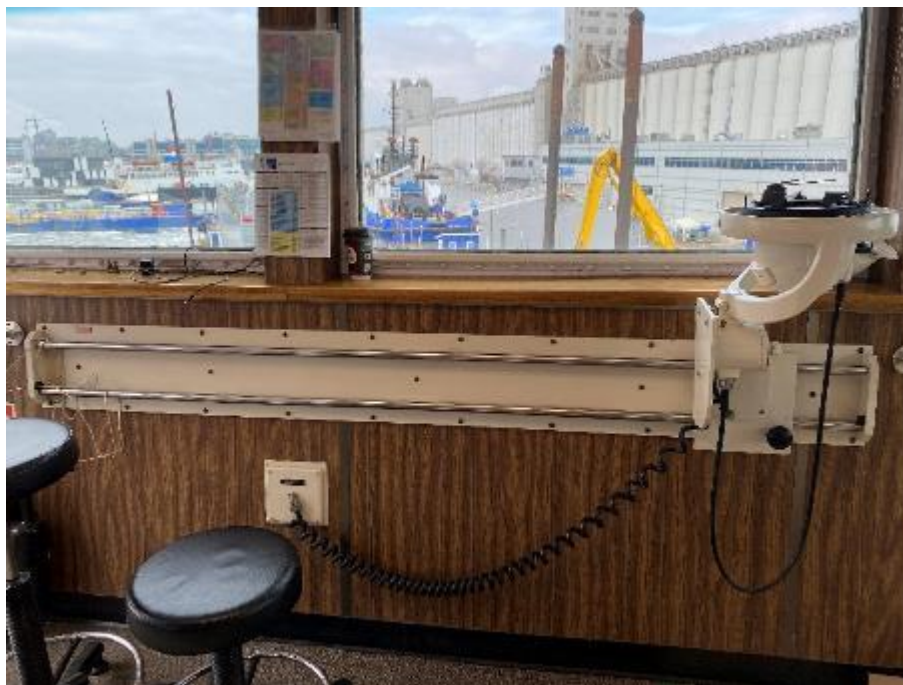
Figure 12: Port Wing Bearing Repeater on rail
