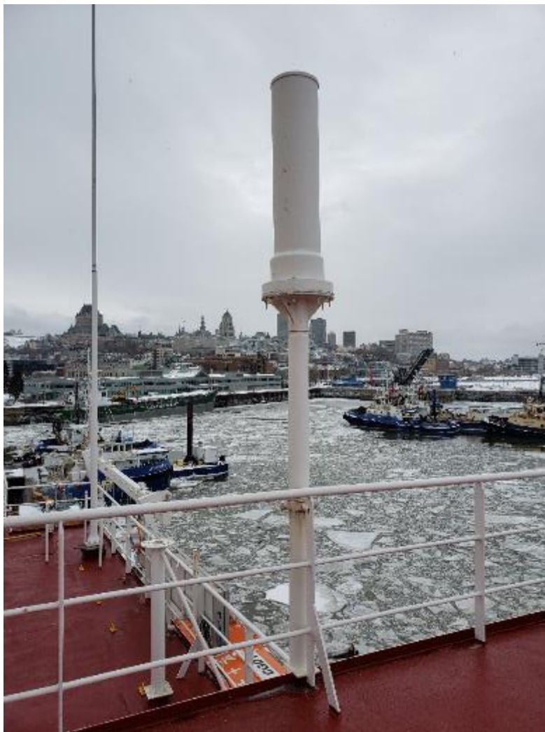
Figure 6: Existing DME Antenna.
