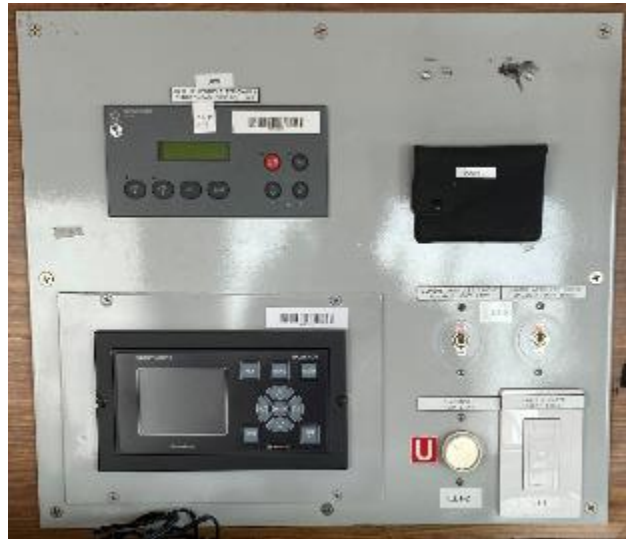
Figure 8: Gyrocompass Operator Unit to be removed
