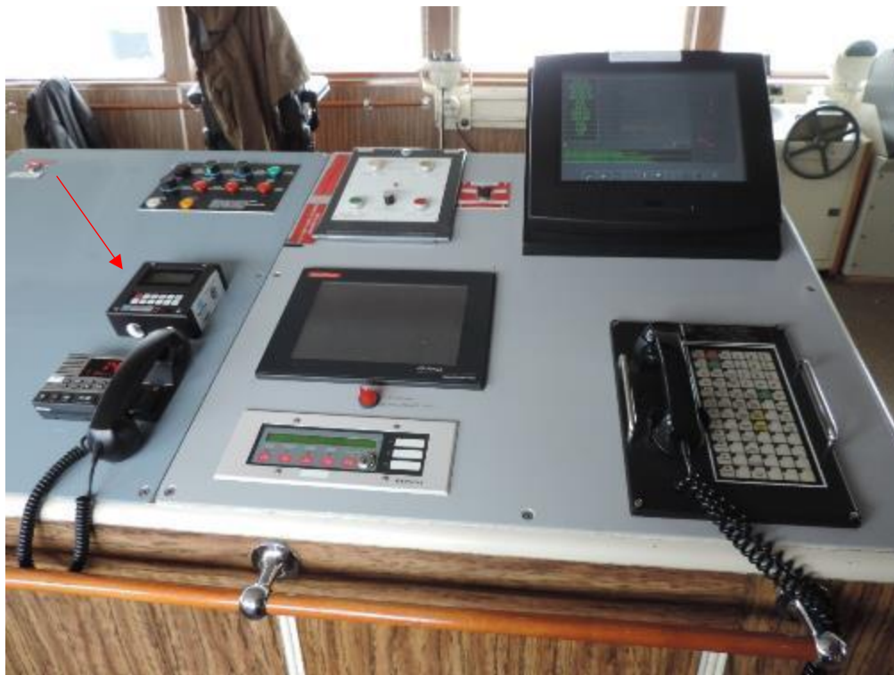
Figure 1: Existing Operator Unit to be replaced with new Bridge Alarm Unit
