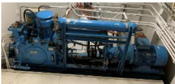
Forward Thruster Hydraulic Power Unit (Fwd Thruster Compartment)
