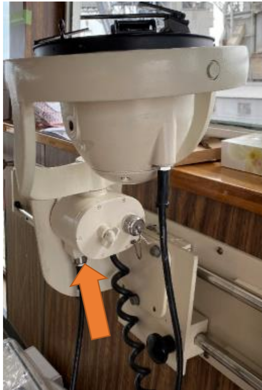
Figure 14: Bearing Repeater Terminal Box
