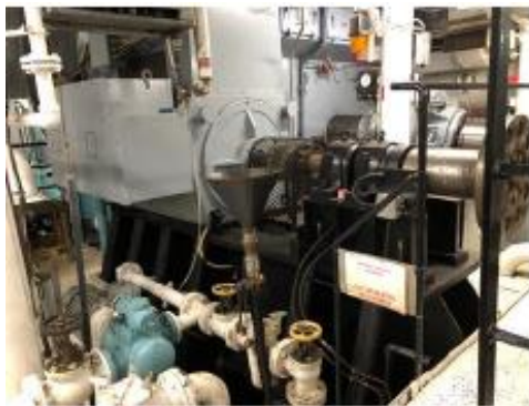
Aft Elettra Electric Drive Motor (Propulsion Motor Room)
