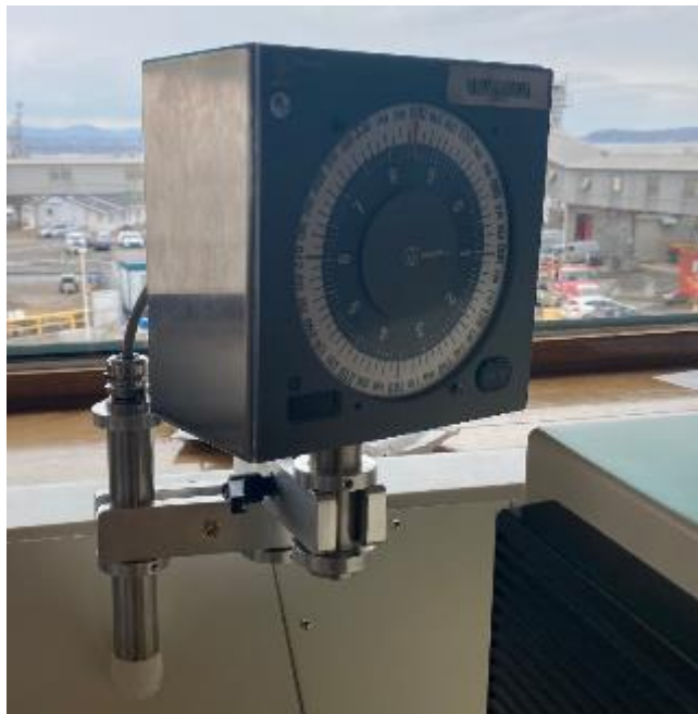
Figure 10: Center Console Steering Repeater to be replaced (Contractor must retain the swivel arm and mounting box in place)
