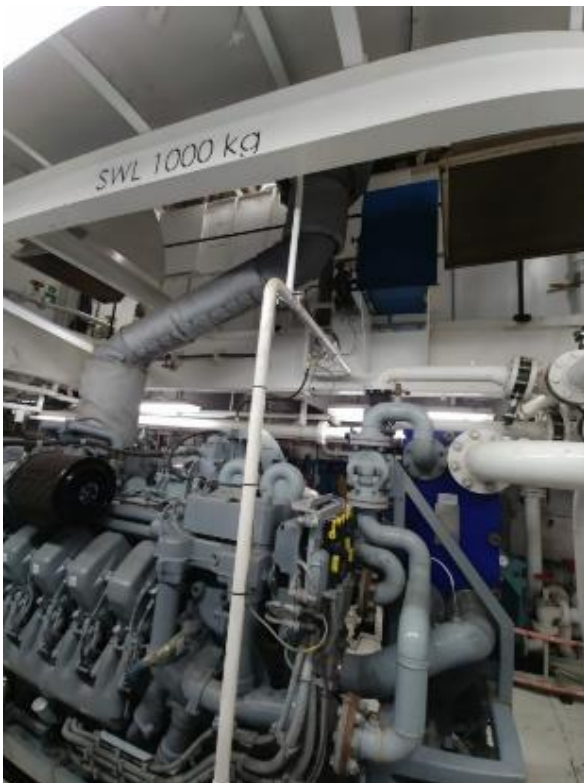
Photo 3 - Expansion tank, its support, piping and eyelets on longitudinal structure
