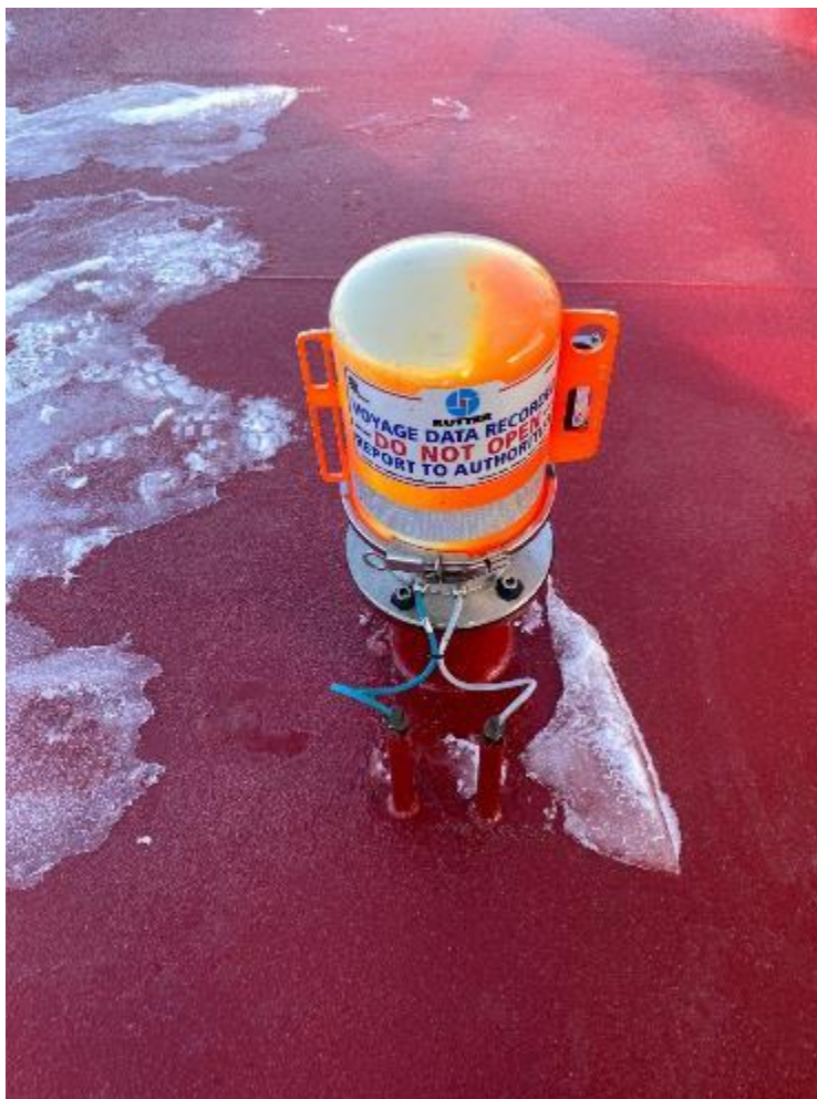
Figure 3 Existing fixed capsule to be replaced. Pedestal to be replaced too.
