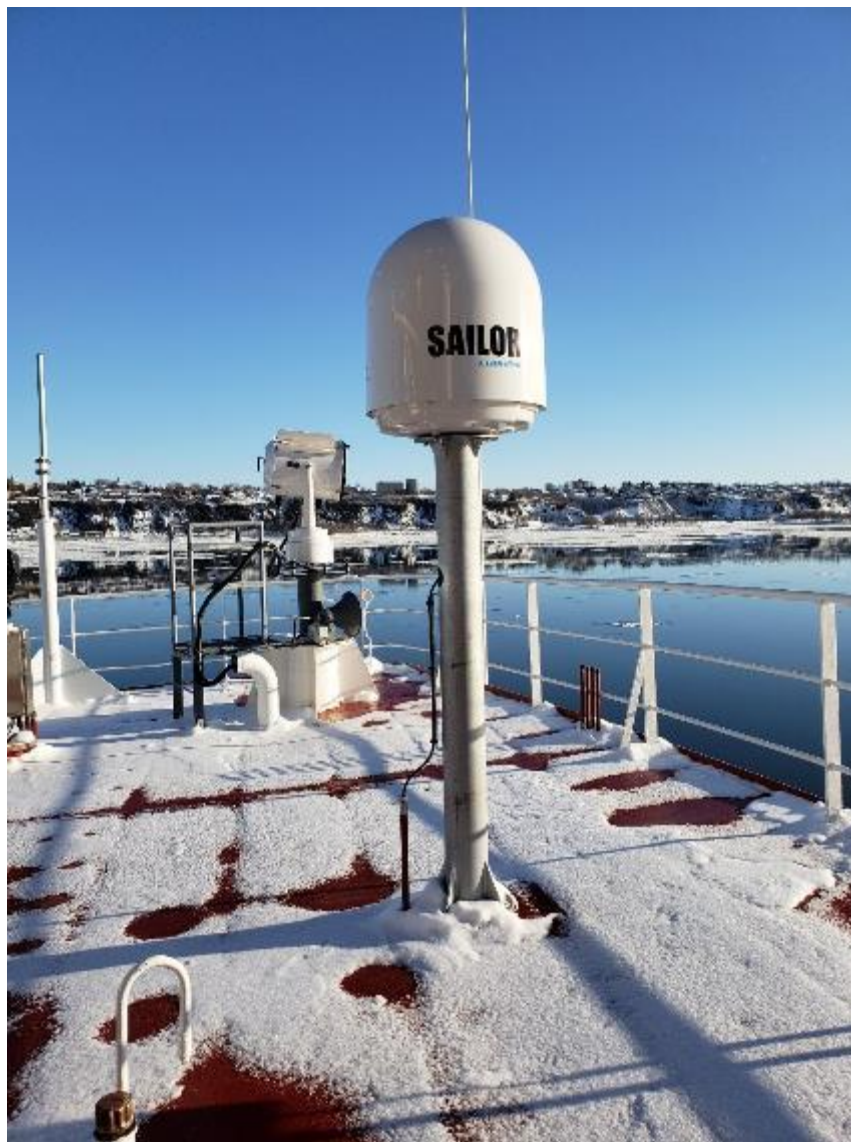
Figure 7: Example of antenna pedestal (NGCC Desgroseilliers)
