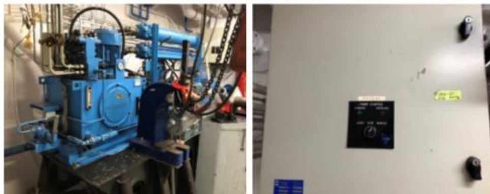
Aft Thruster Hydraulic Power Unit and Control Cabinet (Propulsion Motor Room)
