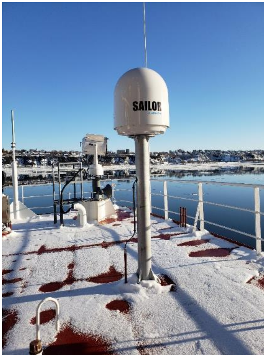
Figure 7: Example of antenna pedestal (NGCC Desgroseilliers)
