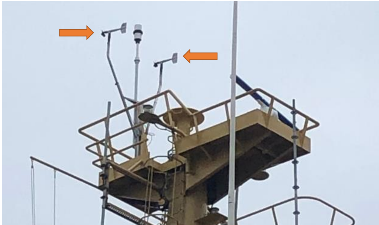
Figure 22: Existing Wind Sensor to be replaced
