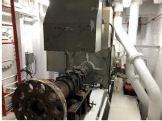
Forward Elettra Electric Drive Motor (Forward Thruster Compartment)
