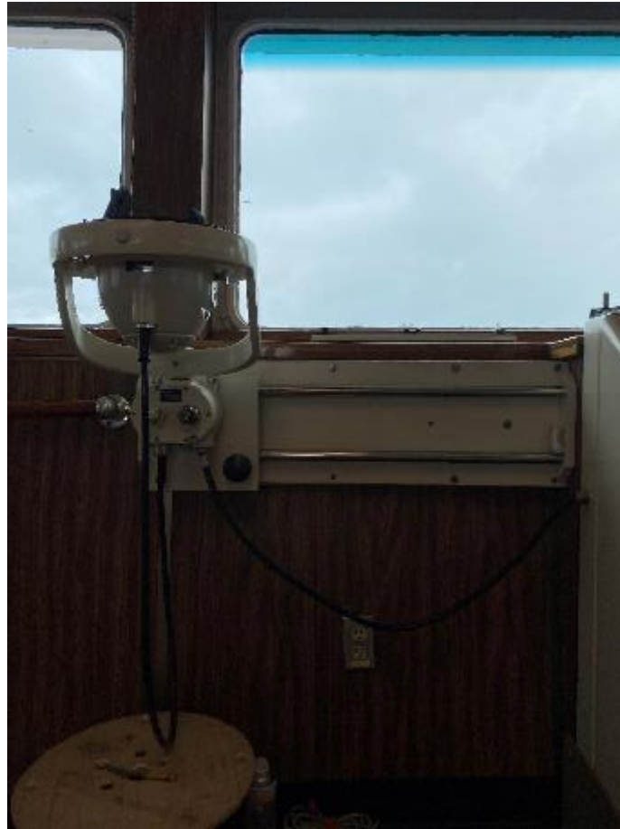
Figure 13: Center Bearing Repeater on Rail
