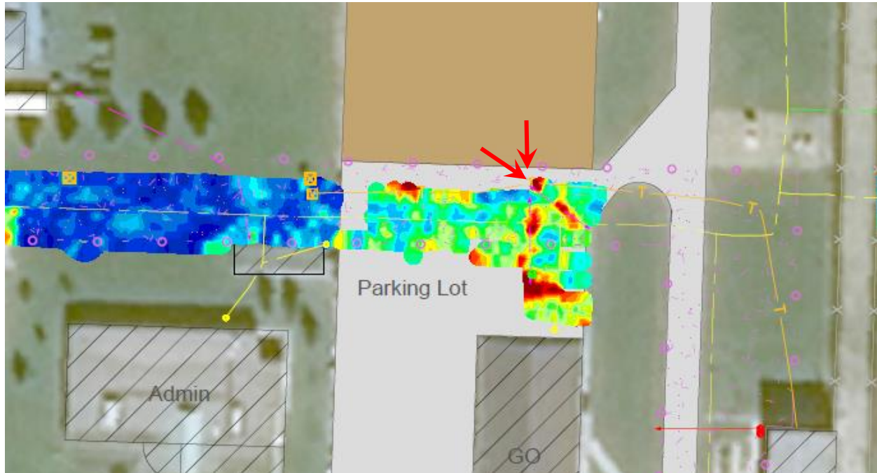
Figure 12: Section of CAD drawing showing buried facilities and GPR reflectivity north of the GO and Admin buildings.
