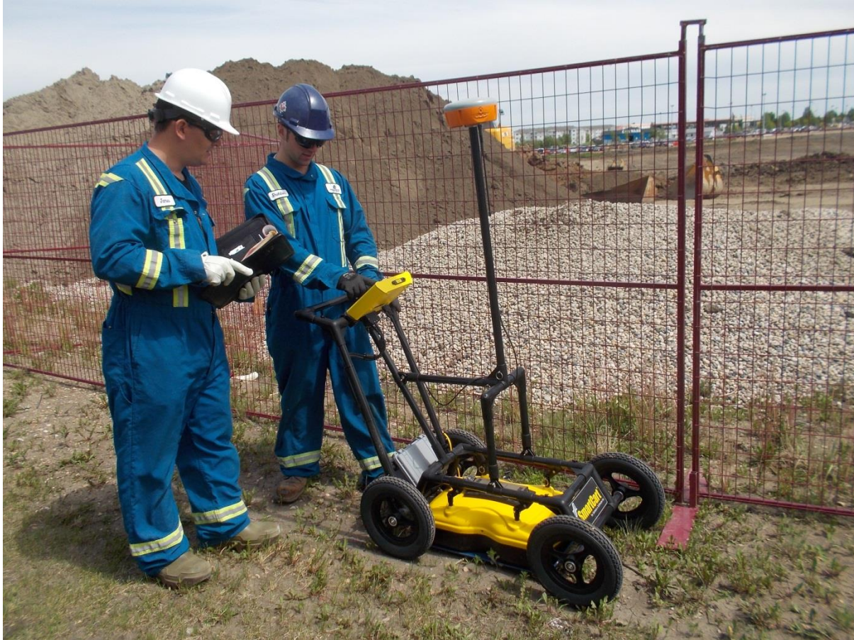
Figure 3: Stock photograph of Maverick Inspection Ltd. technicians using a Noggin250 system deployed with the RTK.
