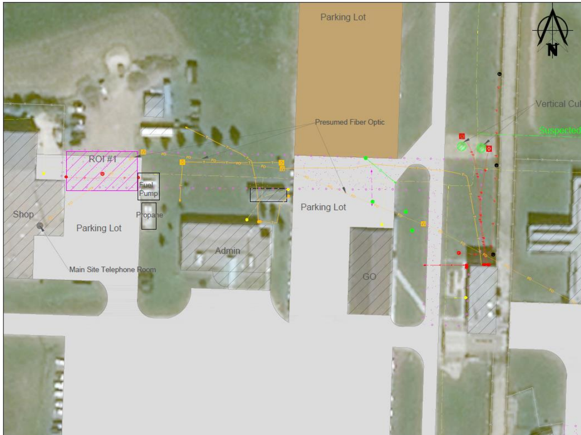
Figure 11: Screen capture of CAD drawing (Page 3) depicting the main outbuilding section with buried facilities and swept area displayed.
