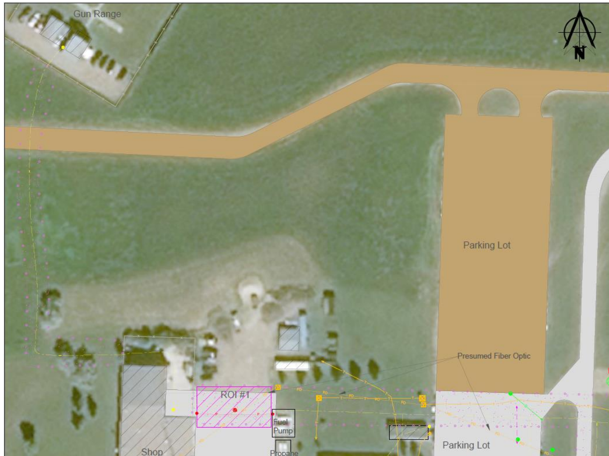
Figure 9: Screen capture of CAD drawing (Page2) showing the northwest detail with buried facilities and swept-area boundaries displayed.
