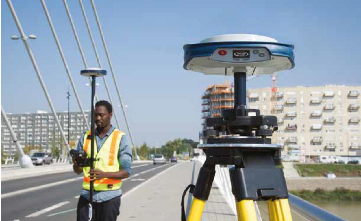
Figure 6: Web-sourced photograph of technician using an SP-80 Ranger connected to the RTK to record locations and positions of detected lines.
