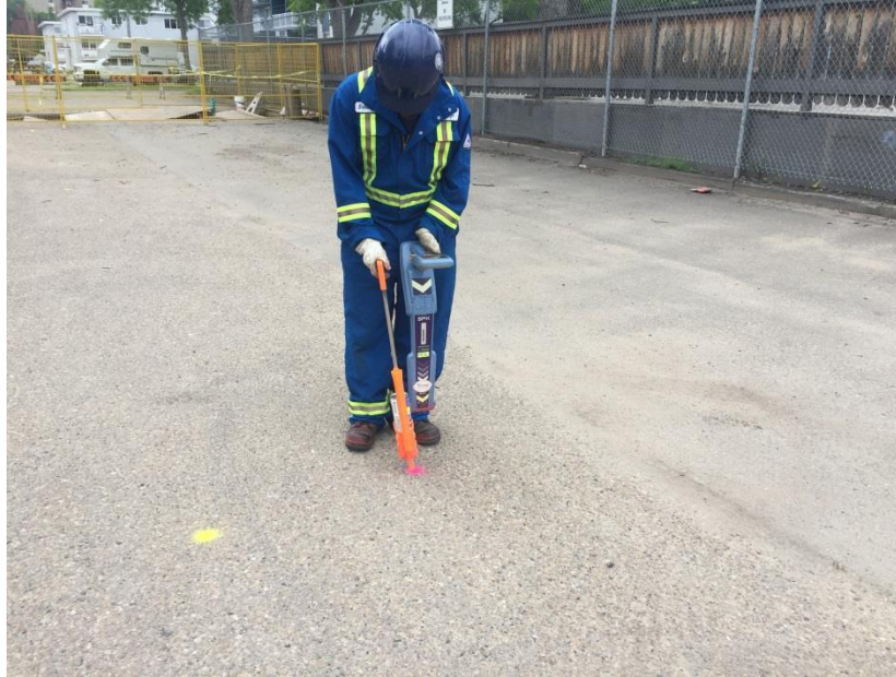
Figure 2: Stock photograph of Maverick Inspection Ltd. technician using an EM Detection utility locator.
