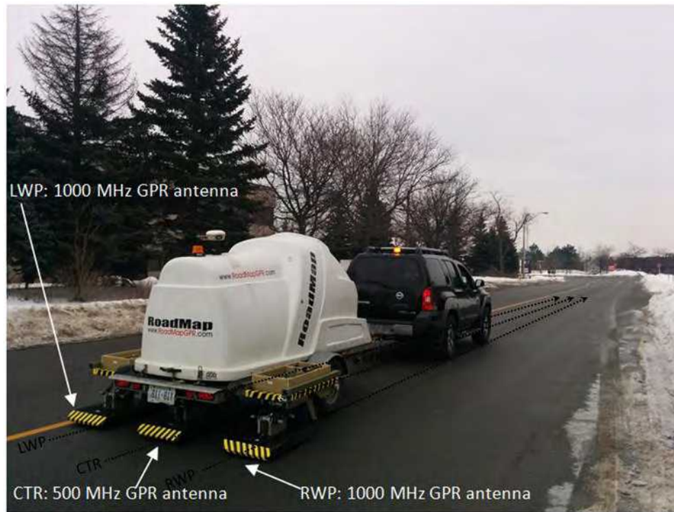
Figure 3-2: Typical RoadMap GPR Acquisition System Setup
