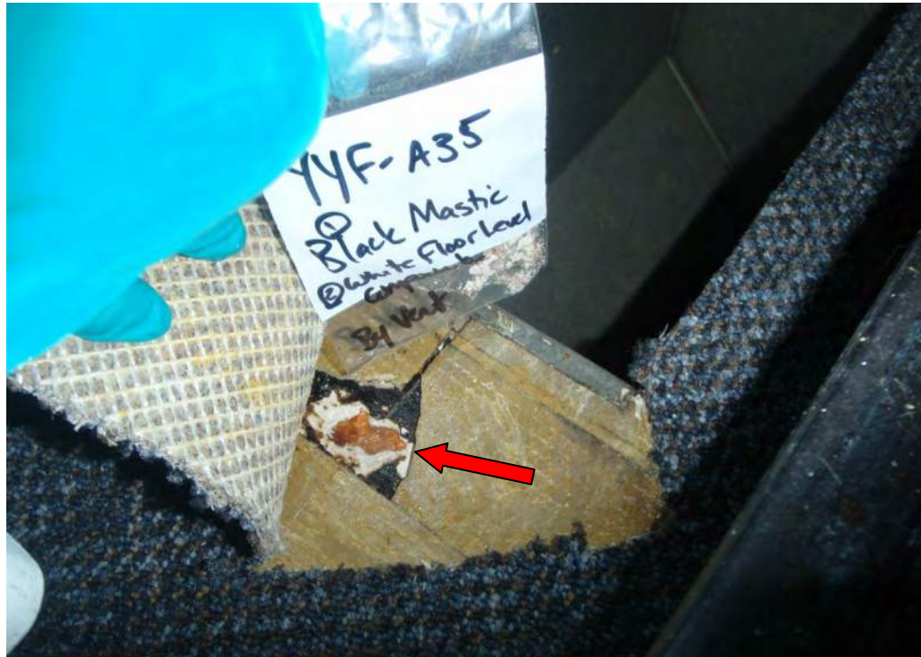
Photograph 37: Asbestos-containing grey vinyl floor tile ( Sample A34 ) and associated black mastic ( Sample A35 ) over white floor leveling compound ( Sample A35 – Layer 2 ) in Room 123.
