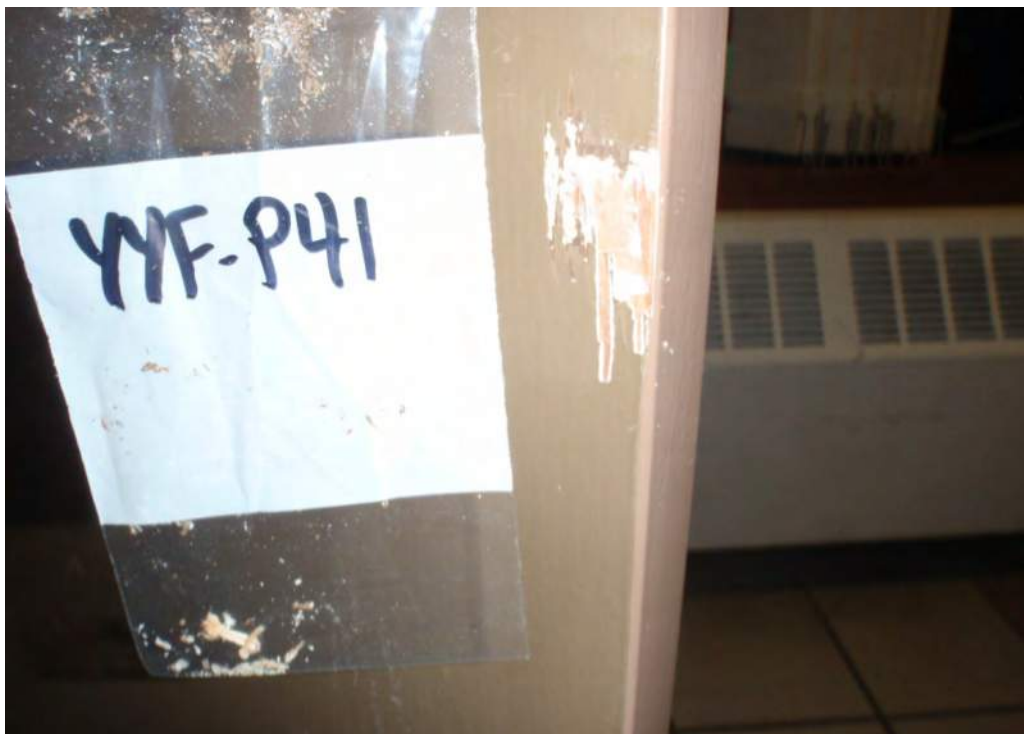
Photograph 84: Lead-based brown paint on door to Room 143 ( Sample P41 ).
