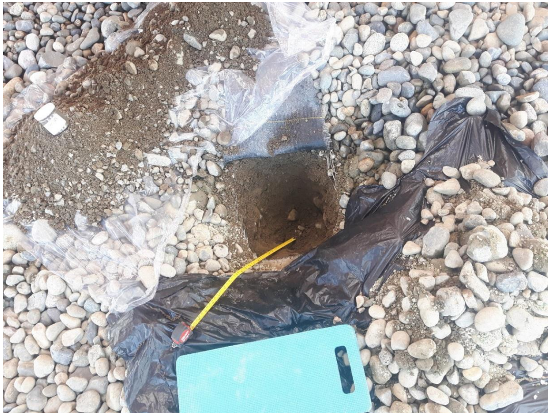
Photo 10: Paddlewheel soil sample 10024-09 at 30 cm depth, sand and gravel, some fines.
