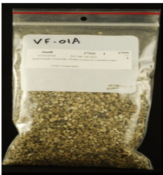
Photo 1 Typical Asbestos-Containing “Small Granule” Vermiculite
