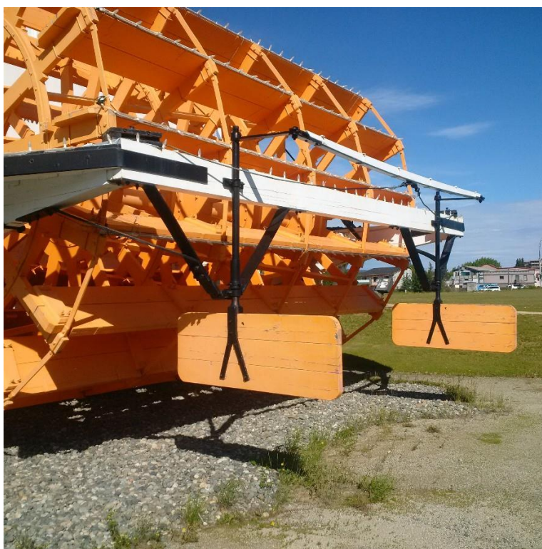
Photo 2: View of Paddlewheel and monkey rudders, facing northwest (away from Yukon river)
