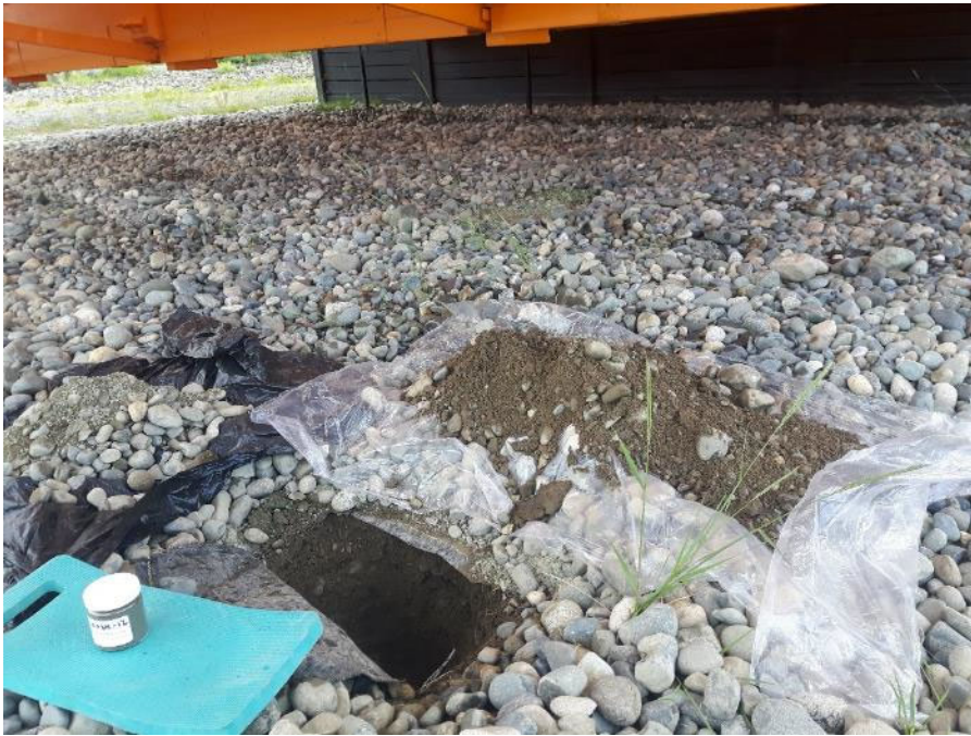
Photo 5: Sample location 10024-12 showing the process of sample collection
