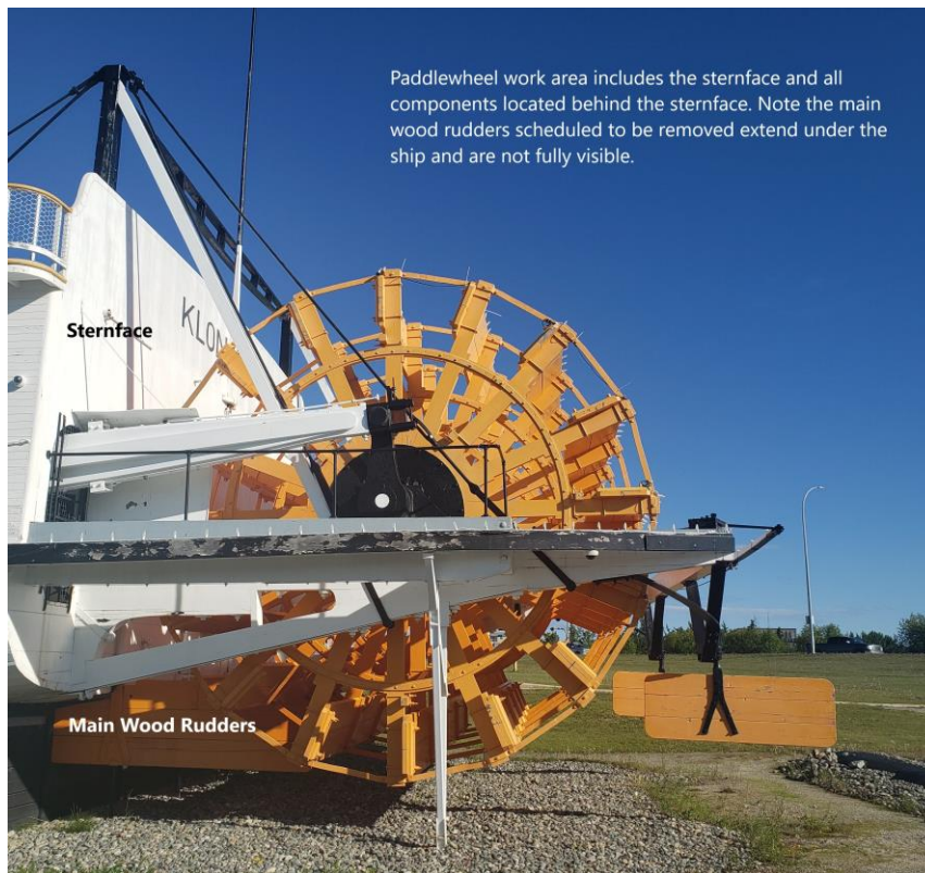
Photo 17: Paddlewheel and associated components lead abatement work area
