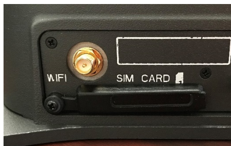
Figure 2-11 Secure the SIM Card Cover
