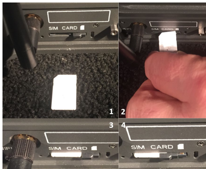
Figure 2-10 Installing SIM Card and Engaging the Lock
