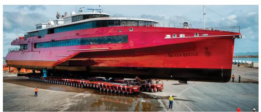
Figure 9 - Trains of SPMT's Moving a Vessel to a Shiplift in Henderson, Australia
