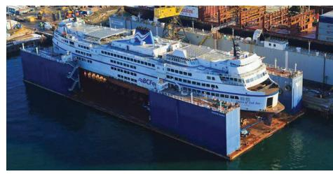
Figure 6 - Floating Drydock (Seaspan Careen) with BC Ferries C-Class Ferry Aboard
