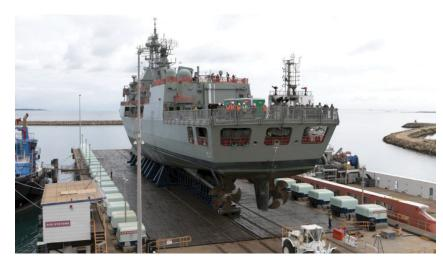
Figure 4 - HMAS Stuart at BAE Systems Henderson Facility, 8,065t Capacity (note tight winch spacing)
