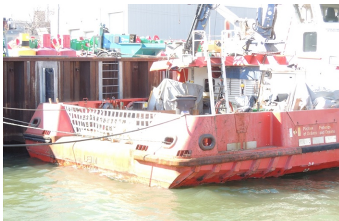
Figure 1: Existing Rub Strake and Trawl Guards (6 Pcs/side) P&S
