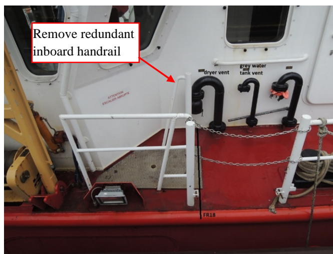
Figure 2: Redundant Handrail. Fo’c’sle Deck, Fr.18
