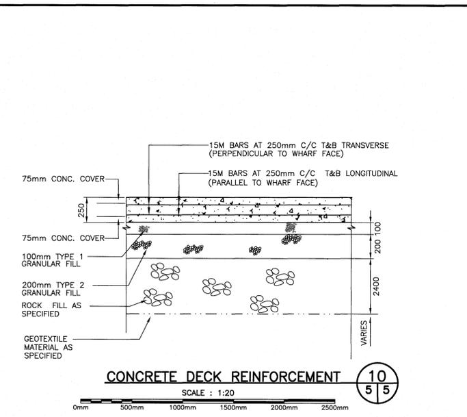
**CONCRETE DECK REINFORCEMENT**
