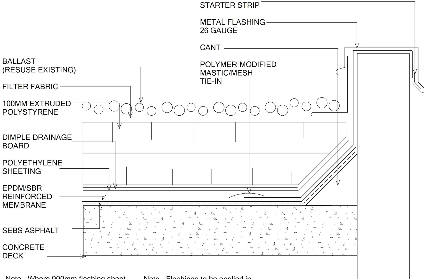
Note - Where 900mm flashing sheet does not extend over outside face of parapet by 75mm. Self adhering membrane must be used to achieve full parapet coverage.
