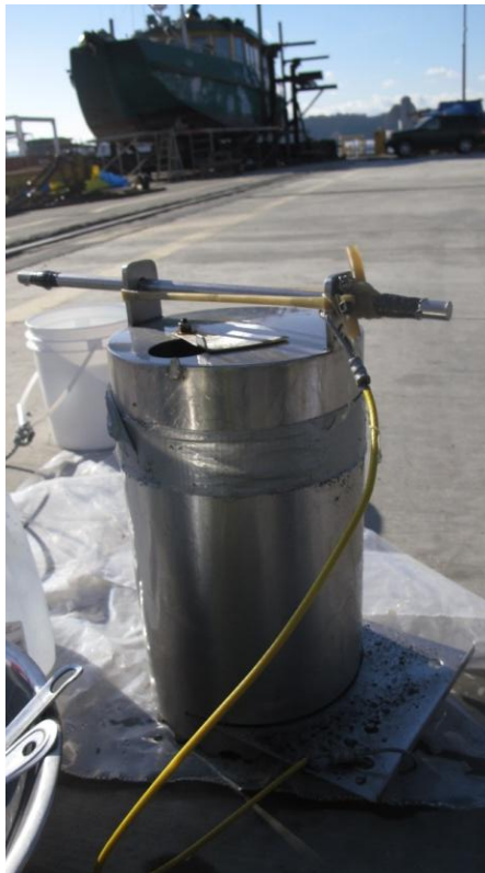
Photograph 3: Stainless steel grab sampler provided by RSS.
