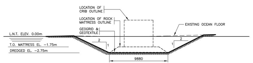
**SECTION - DREDGE - PHASE 1 AT HEADER CRIB**
