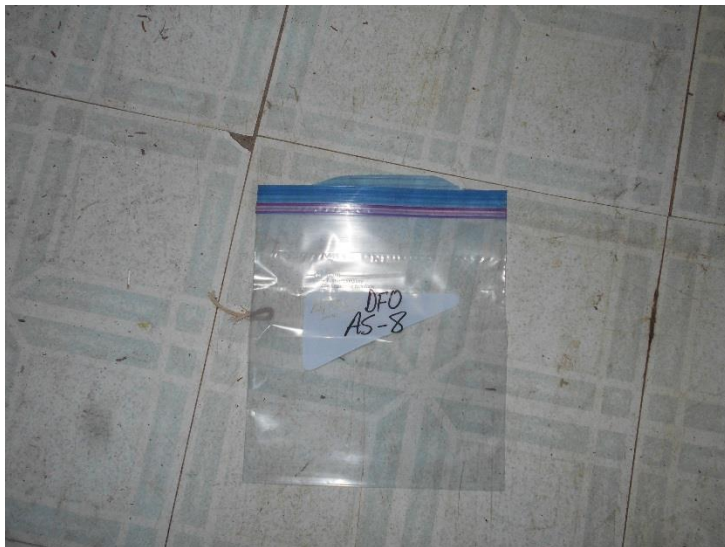
Photo 16 - View of bulk sample CA-AS-8 (green square pattern vinyl floor tile).
