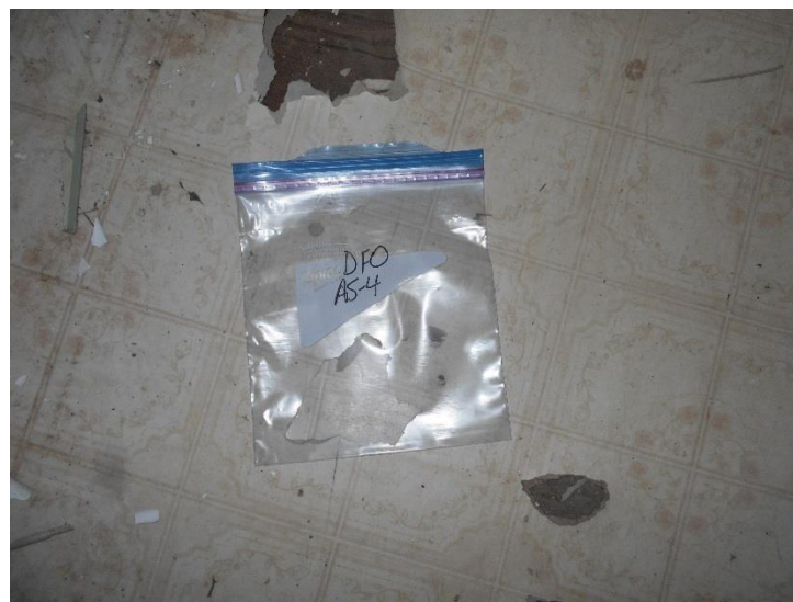
Photo 12 - View of bulk sample CA-AS-4 (beige and brown pattern vinyl sheet flooring).
