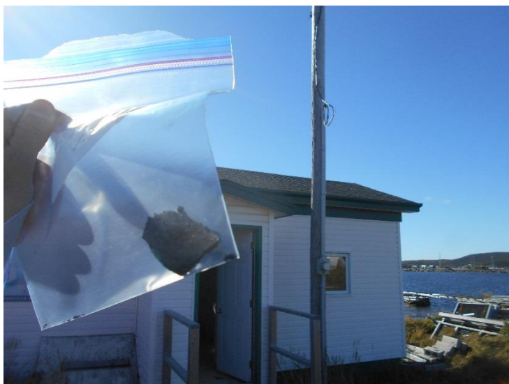
Photo 9 – View of bulk samples CA-AS-1 (black asphalt shingle).
