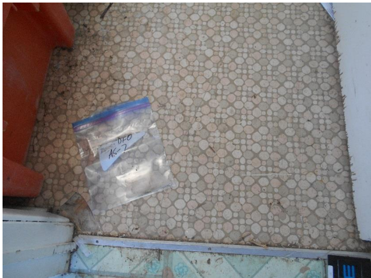
Photo 15 - View of bulk sample CA-AS-7 (beige pebble pattern vinyl sheet flooring with brown mastic).
