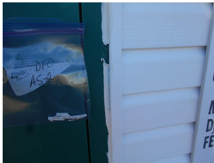
Photo 10 – View of bulk sample CA-AS-2 (white caulking).
