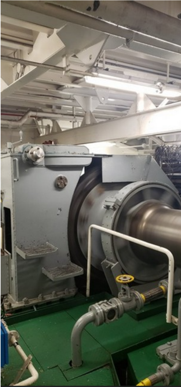
Photo 6 – port side turning gear (looking aft towards starboard side-outboard)
