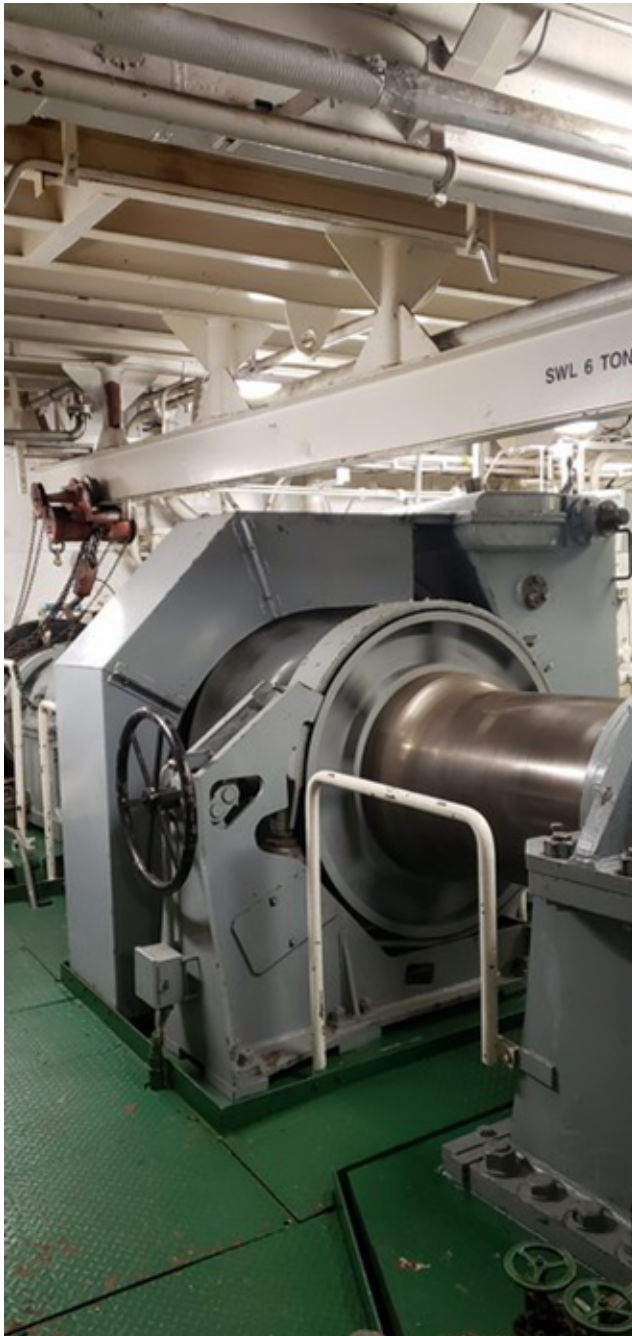
Photo 12 – Starboard turning gear (looking aft towards port side-inboard)
