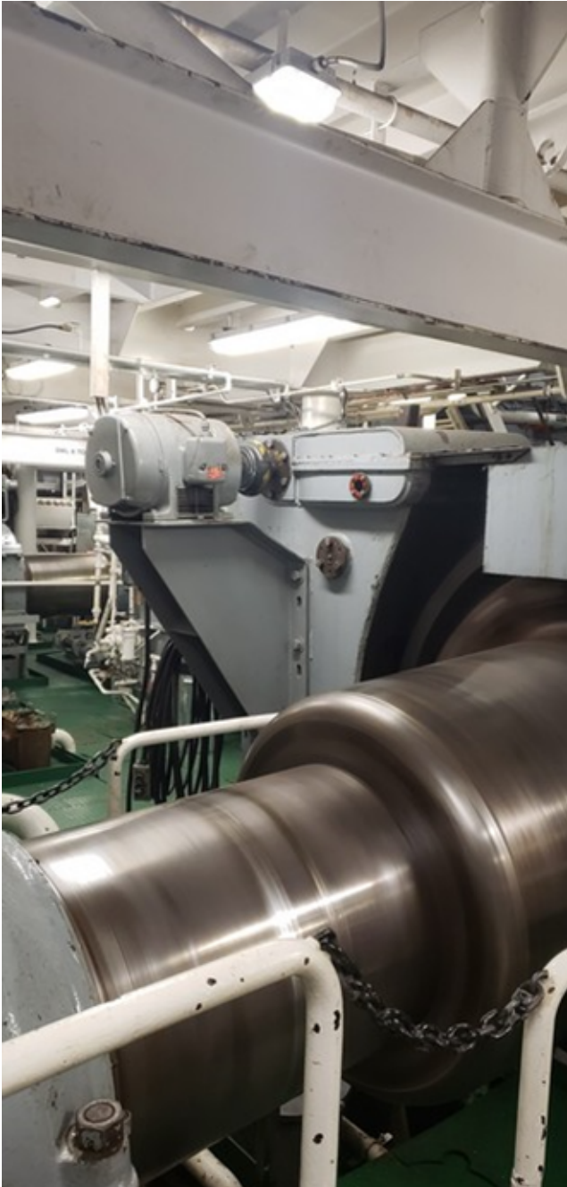
Photo 9 – starboard turning gear (looking forward towards port side-inboard)
