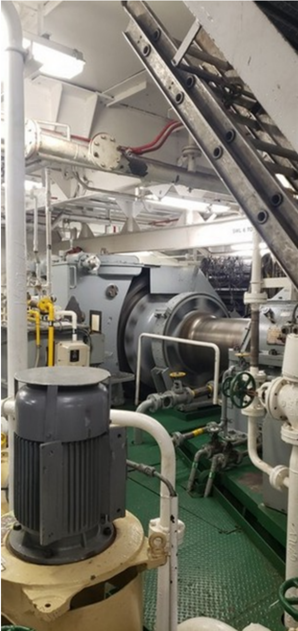
Photo 5 – port side turning gear (looking aft towards starboard side-outboard)
