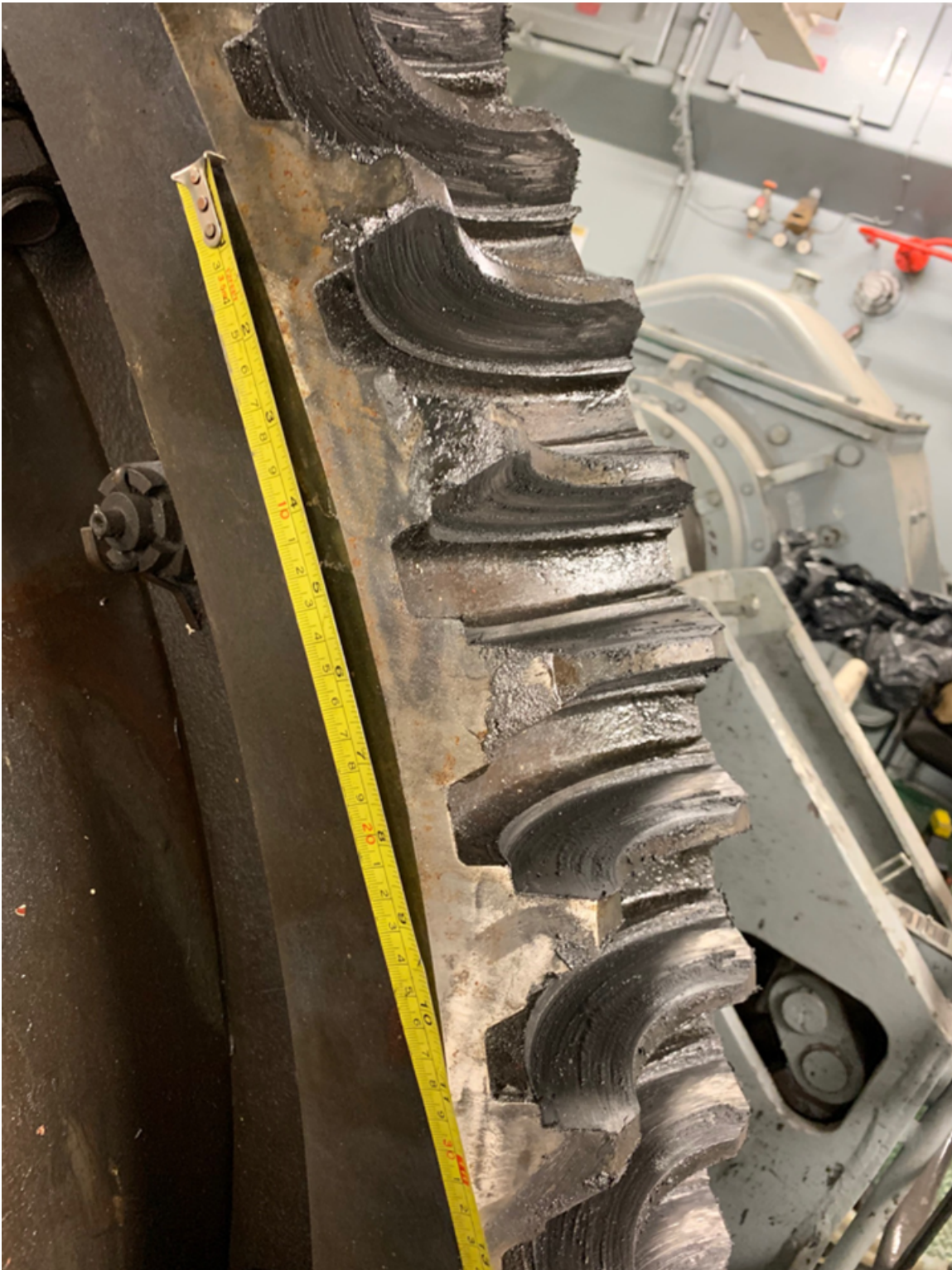
Photo 2 – Starboard side cast iron gear wheel wear
