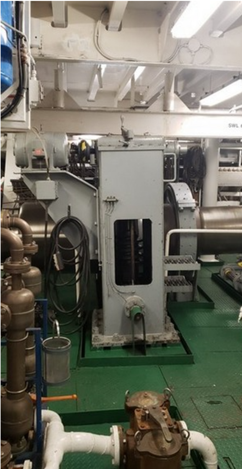
Photo 8 – port side turning gear (looking midships towards starboard side-outboard)
