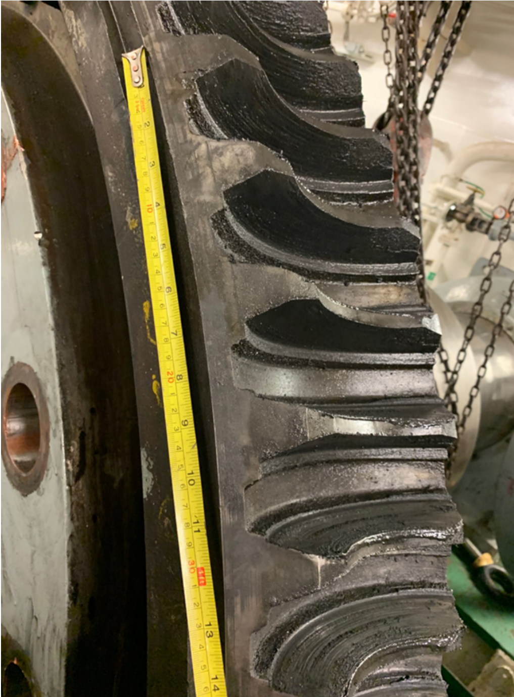
Photo 1 – Port side cast iron gear wheel wear
