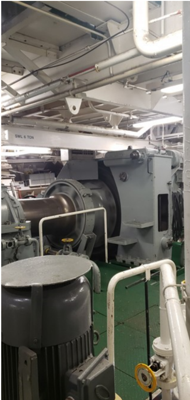
Photo 11 – Starboard turning gear (looking aft towards starboard side-outboard)
