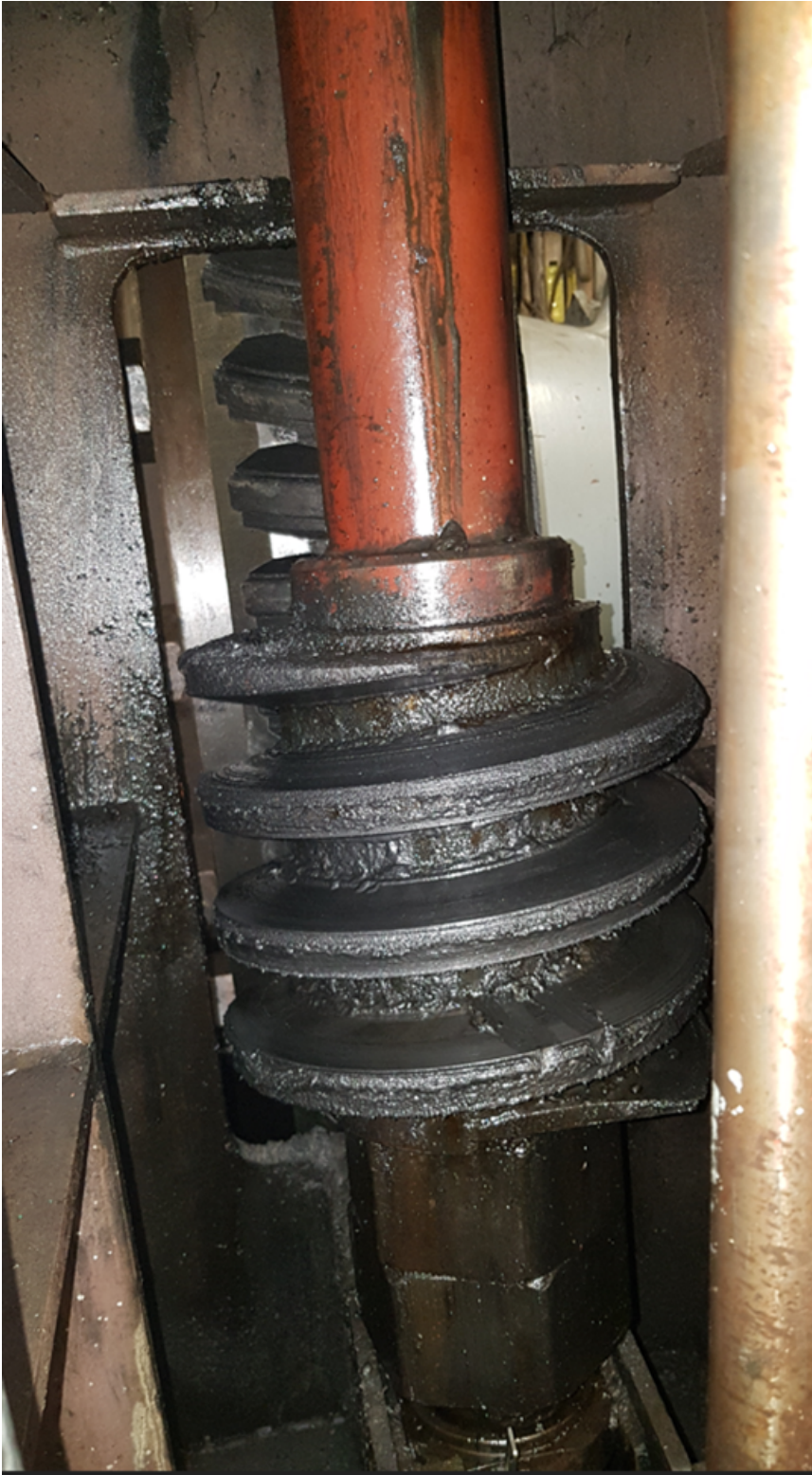
Photo 3 – Port side worm gear as viewed through access way (starboard side is identical)
