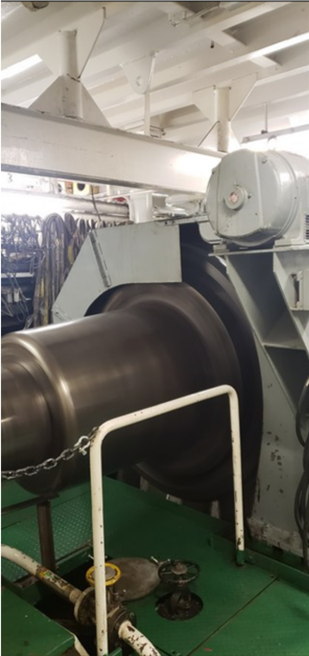
Photo 4 – Port side shaft turning gear (looking forward towards starboard-outboard)
