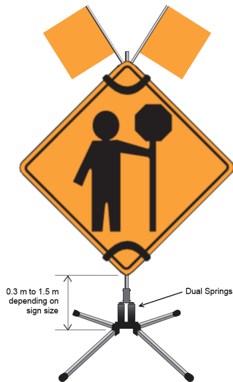
Figure 02: Wind Resistant Sign Stand
