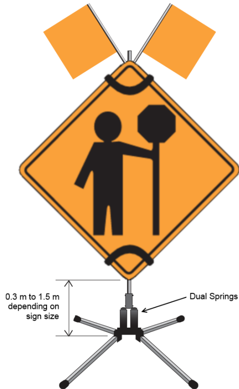
Figure 01 35 00 - 02: Wind Resistance Sign Stand
