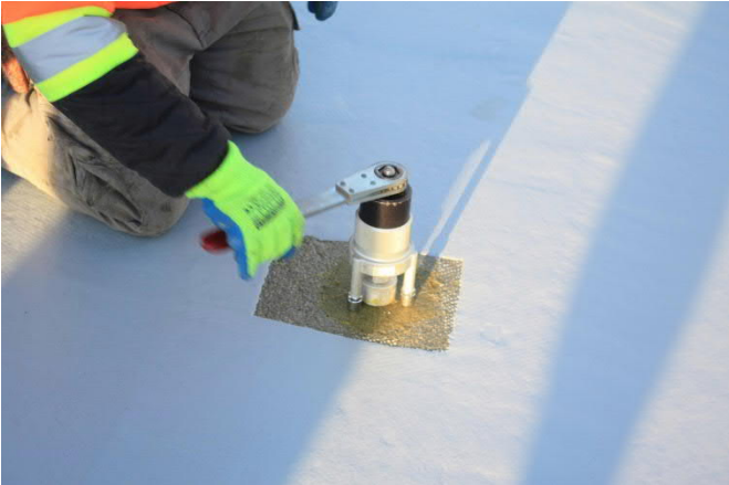
Figure 23: Test to ensure adequate bond between concrete and Matacryn bonding agent
