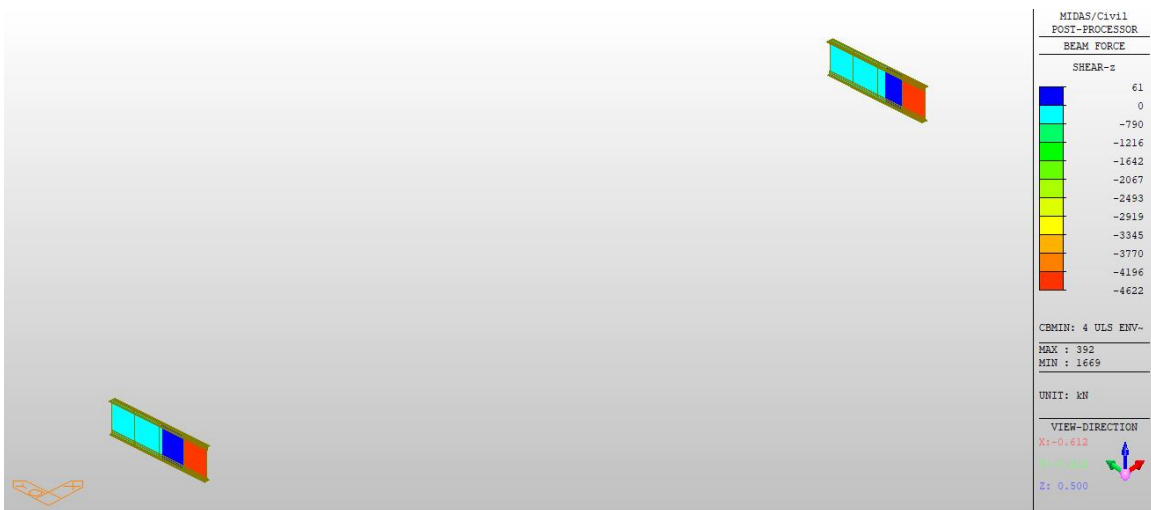
Figure 90 Lift Girder Case 4 ULS F_z Min
