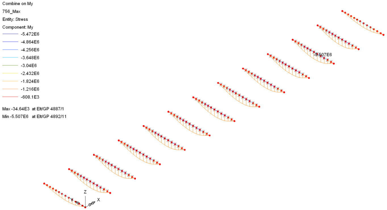
Figure C03: Lift Span Floor Beams - Maximum Moment
