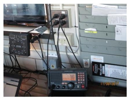
Photo E19 Wind Speed Indicator and Marine Radio. Both units are of the existing installation and are in good serviceable condition.
