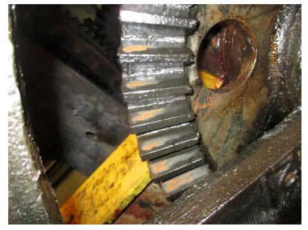
Photo M8 Gearset G2/P2-SE, Differential Gear. There was corrosion on some of the differential gear teeth due to inadequate lubricant
