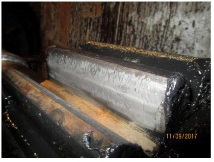
Photo M7 G1-SW-OB. Damage to the gear tooth caused by wire intrusion is wearing in.
