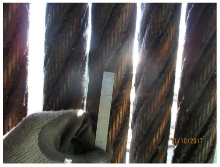
Photo M18 NW-IB Counterweight Ropes. The maximum counterweight rope wear flats were measured to be 5/8".
