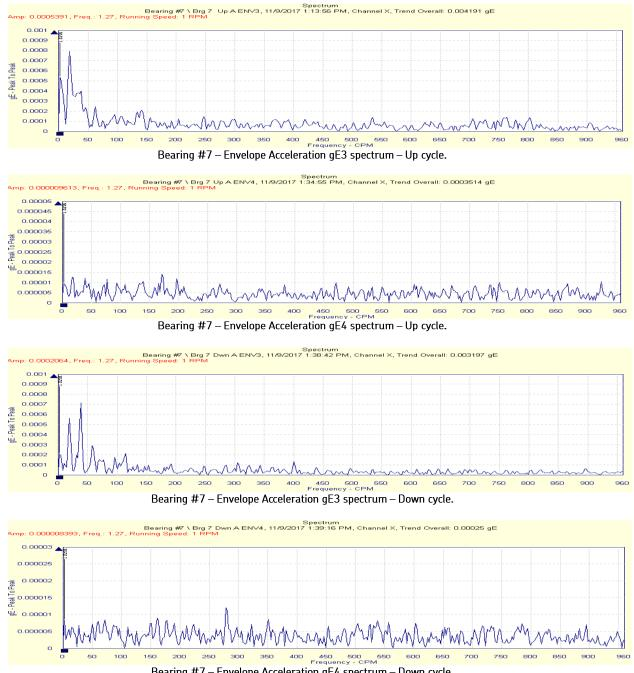
Bearing #7 – Envelope Acceleration gE4 spectrum – Down cycle.
