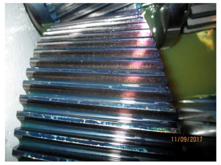
Photo M11 South Span Drive Reducer Auxiliary Gears. The reducer gear teeth have minor damage that may be from particles passing through the mesh.
