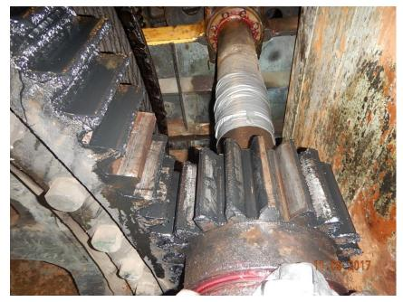
Photo M6 Pinion P1-SW-OB. The gear teeth in the acceleration zone were cleaned to bare metal for inspection. Gear tooth thickness measurements were taken at all gears.
