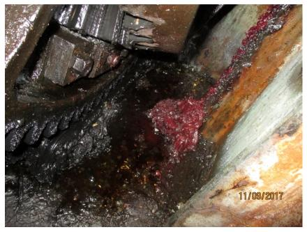
Photo M9 G2/P2-SE, Support Frame. There was an accumulation of old grease within the support frame under the G2 gear.
