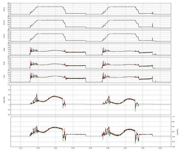
Figure E3: Voltage, Current, and Power Parameters (South Tower East Span Drive Motor – Normal Power)
