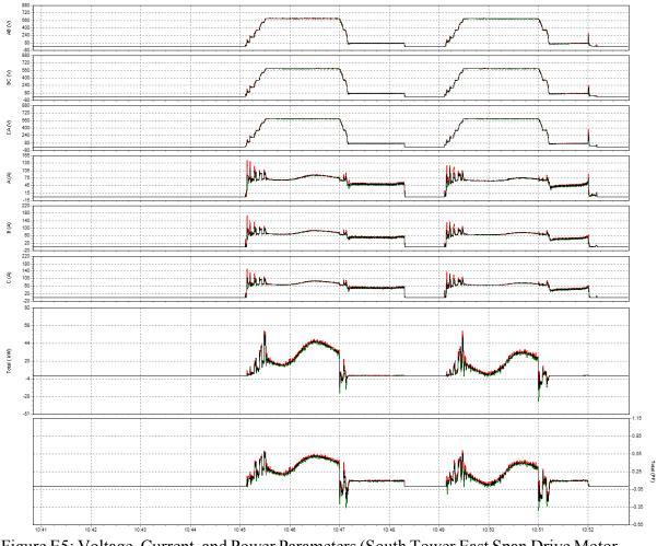
Figure E5: Voltage, Current, and Power Parameters (South Tower East Span Drive Motor on Generator Power)
