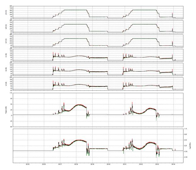
Figure E2: Voltage, Current, and Power Parameters (North Tower West Span Drive Motor – Normal Power).
