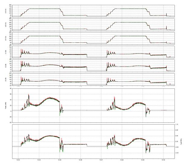
Figure E4: Voltage, Current, and Power Parameters (North Tower East Span Drive Motor – Normal Power).
