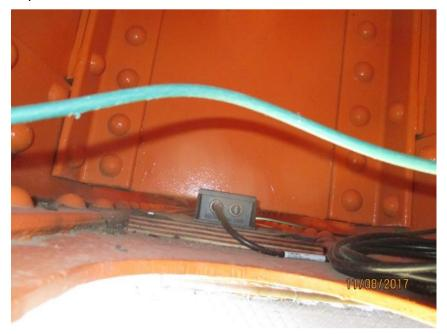
Photo E40 Inclinometer Unit. The span inclinometer had been moved several times under the direction of the Engineer during the rehab project. The function of the inclinometer
