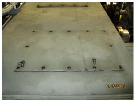
Photo M13 North Span Drive Reducer. The inspection cover screws have damaged threads.
