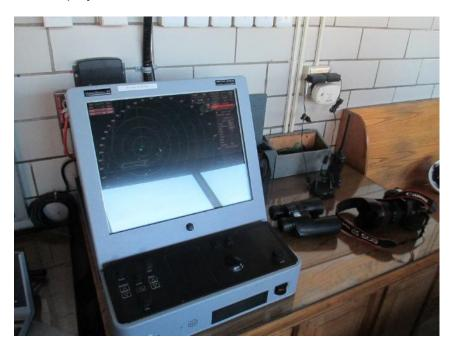
Photo E18 Bridge Radar System. The Radar system was installed to aid the bridge operation and schedule for the boat traffic. It also capable of display the wind speed and direction.
