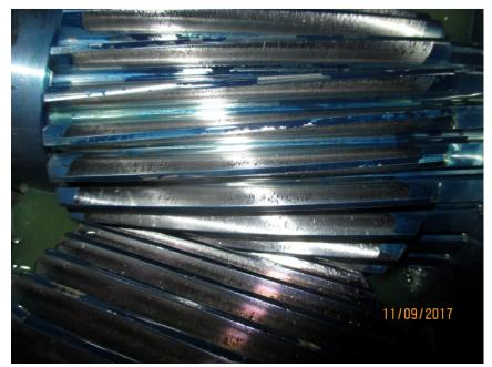
Photo M10 South Span Drive Reducer Auxiliary Gears. The reducer gear teeth have minor damage that may be from particles passing through the mesh.
