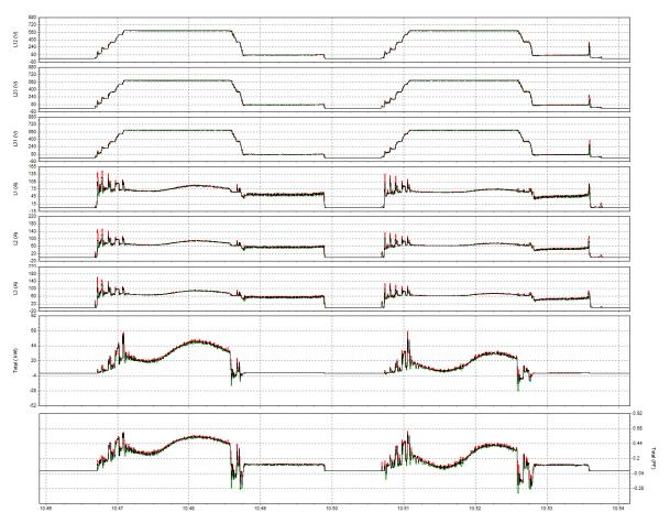
Figure E6: Voltage, Current, and Power Parameters (North Tower East Span Drive Motor on Generator Power).
