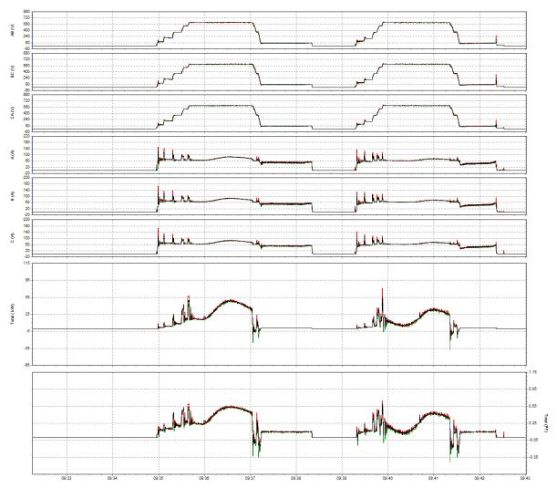
Figure E1: Voltage, Current, and Power Parameters (South Tower West Span Drive Motor – Normal Power)
