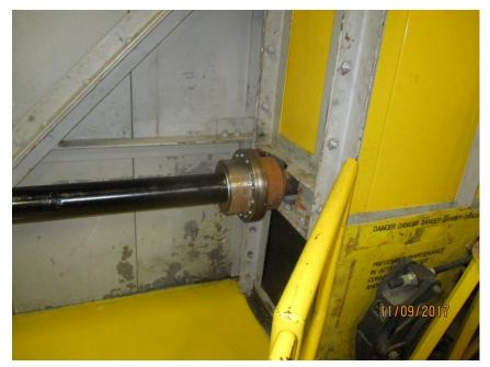
Photo M4 Coupling C1-SE. There was light corrosion on the hub. Corrosion was noted at all C1 and C2 couplings.
