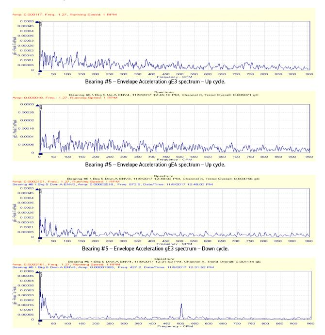
Bearing #5 – Envelope Acceleration gE4 spectrum – Down cycle.
