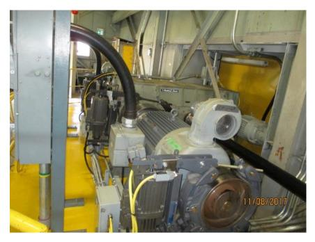
Photo E24 Typical Drive Machinery Arrangement. The span motors and motor brakes are in as-new condition. The machinery brakes are existing but are provided with a new brake drum.
