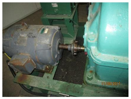
Photo M28 South Span Lock Machinery. Several components including the shaft and bolts are not fully painted. A coating of rust inhibitor limits corrosion.
