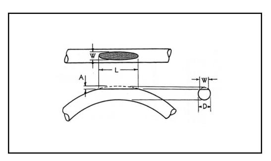
FIGURE 5 – Illustration of Elliptical Wear Area
