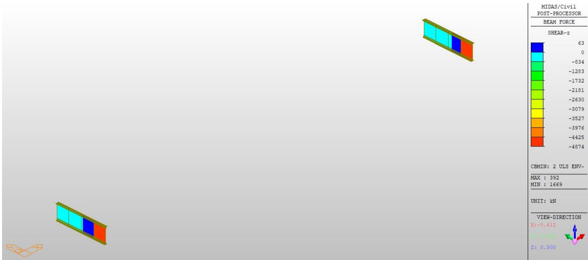
Figure 42 Lift Girder Case 2 ULS F z Min
