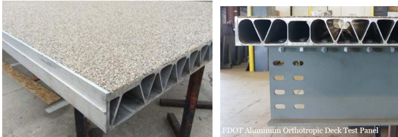
Figure 12: Aluminum decking with wearing surface 2,12
