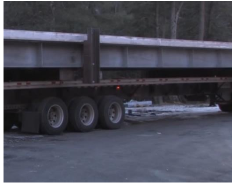
Figure 1: Deck on stringer shipping
