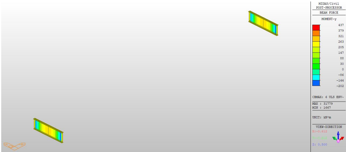
Figure 135 Lift Girder Case 6 ULS M_y Max
