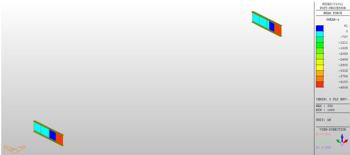
Figure 66 Lift Girder Case 3 ULS F z Min
