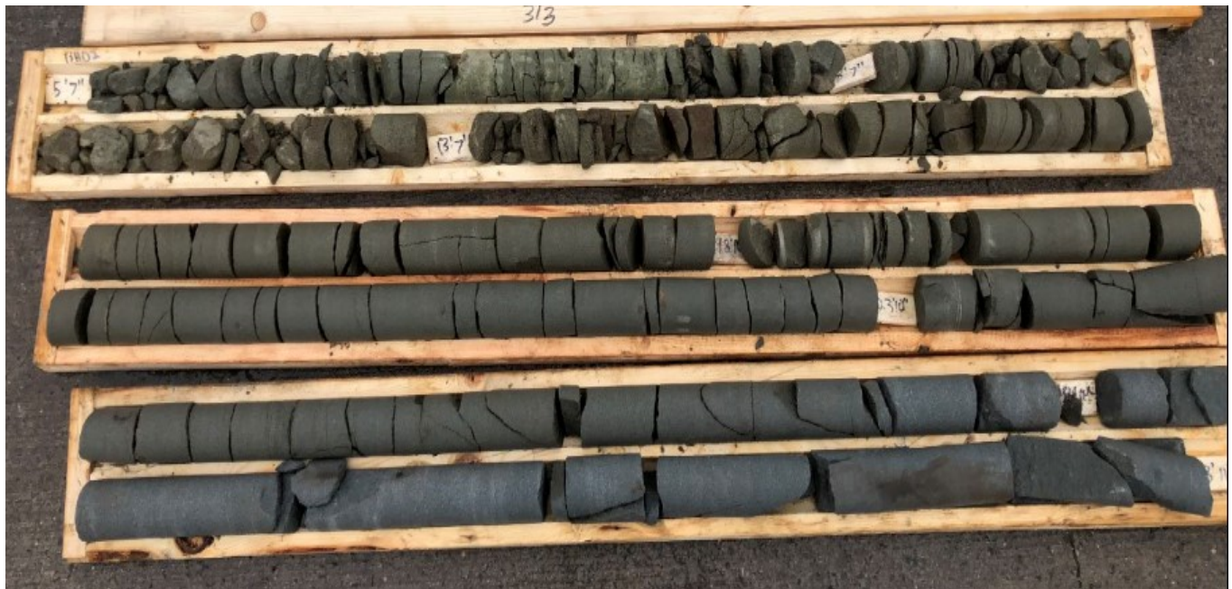
Photo 2: BH-18-02 Seabed Elevation : -2.0 meters Bedrock Elevation : -2.3 meters Amount cored : 10.1 meters
