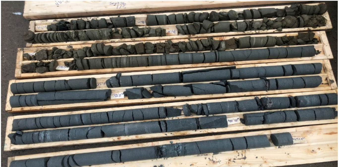
Photo 3: BH-18-03 Seabed Elevation :-1.5 meters Bedrock Elevation :-2.1 meters Amount cored : 13.4 meters
