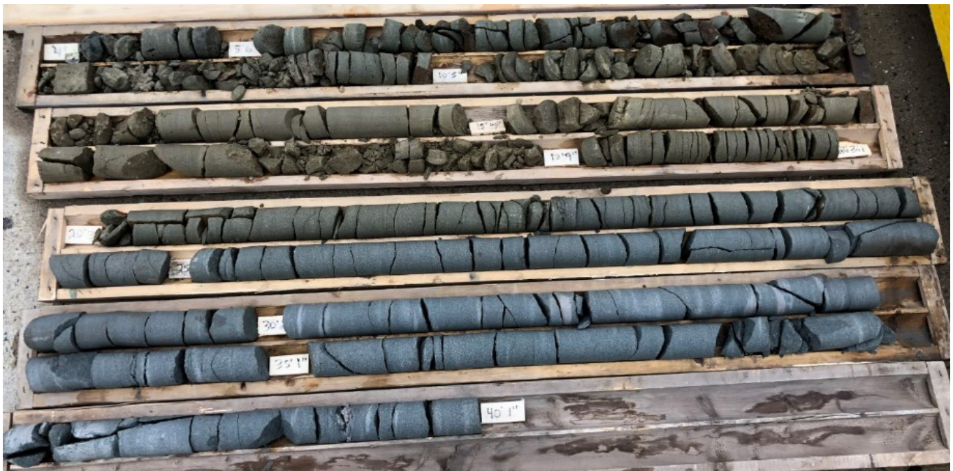
Photo 4: BH-18-04 Seabed Elevation :-1.7 meters Bedrock Elevation :-2.1 meters Amount cored : 11.8 meters
