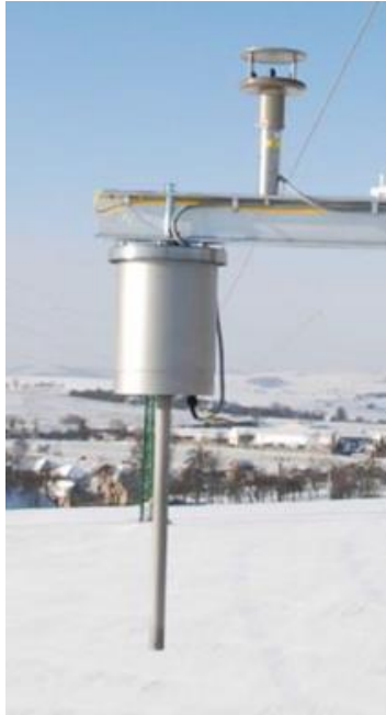
Figure 6-9 An example of wind and ice sensors installation
