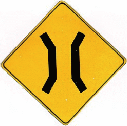
(a) Narrow Structure Sign
