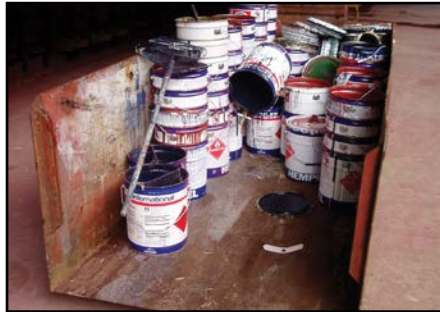
Residual paint in the cans may drip out of the skip and enter the marine environment through the drain systems.
