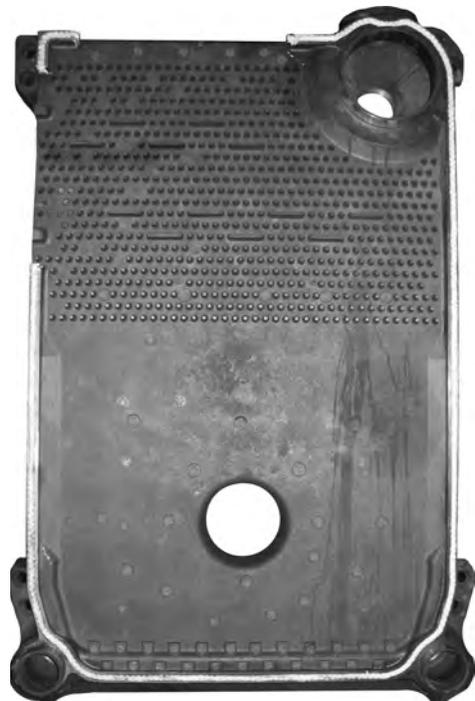
**Figure 7: Affixing the Fiberglass Rope**
