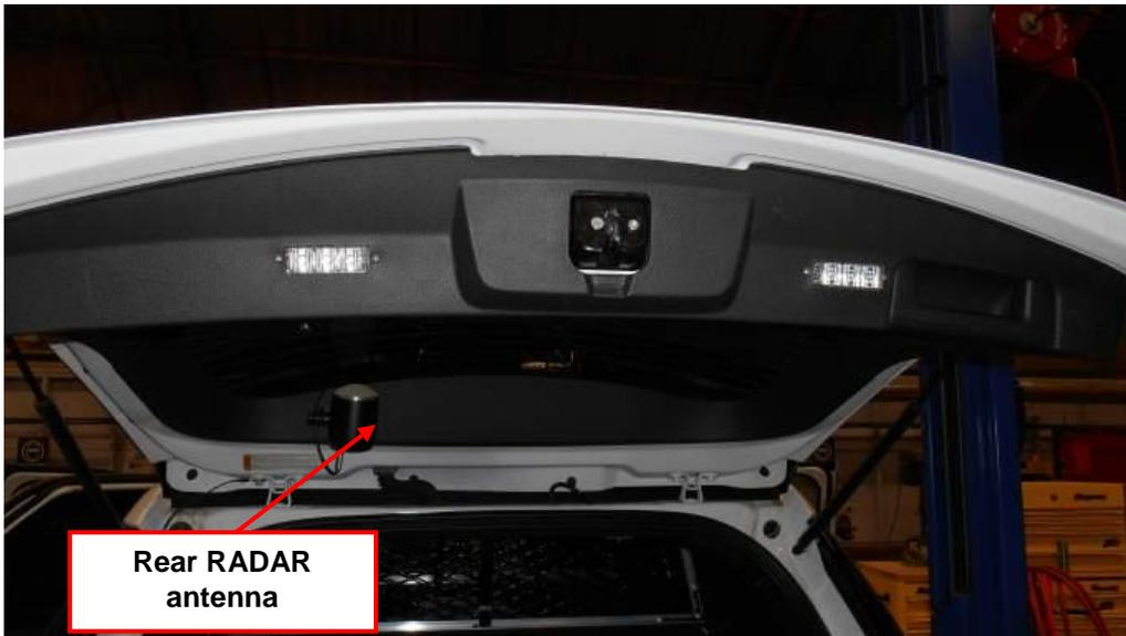
**FIGURE 12C – Rear RADAR antenna location**
