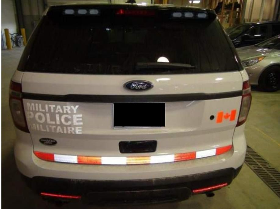
**FIGURE 5A –Rear view - Alternate rear conspicuity marking**
