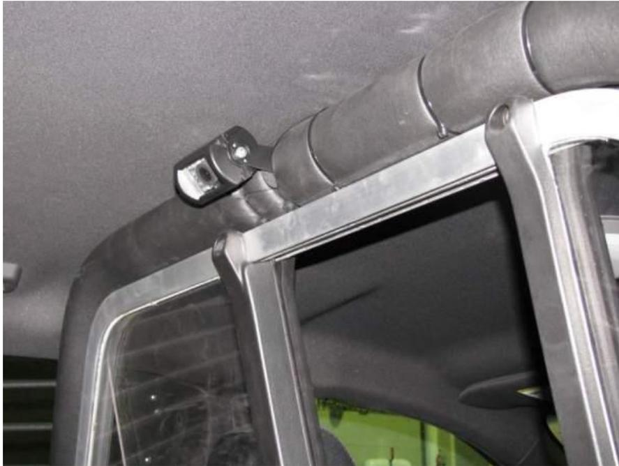
**FIGURE 19 – MVRS rear camera**
