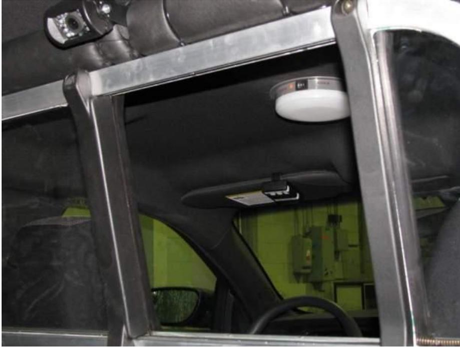
**FIGURE 21– Security screens (with sliding center window and MVRS rear camera)**
