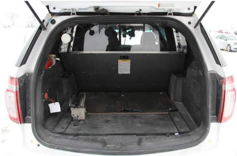
***FIGURE 24 – Example of the approved cargo barrier installation in an SUV-type marked MP vehicle***
