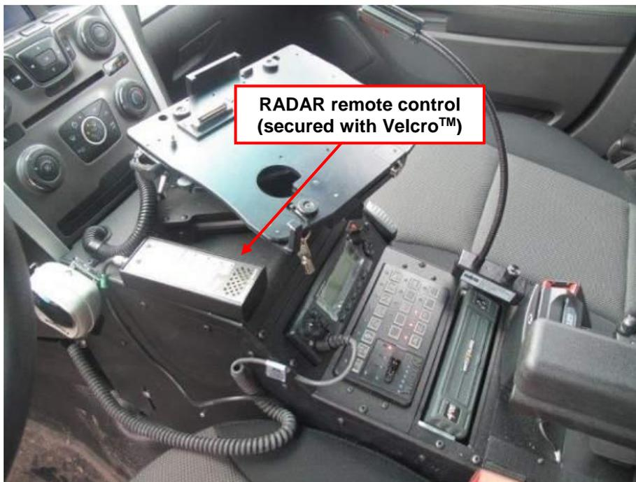
**FIGURE 14– RADAR remote control location**
