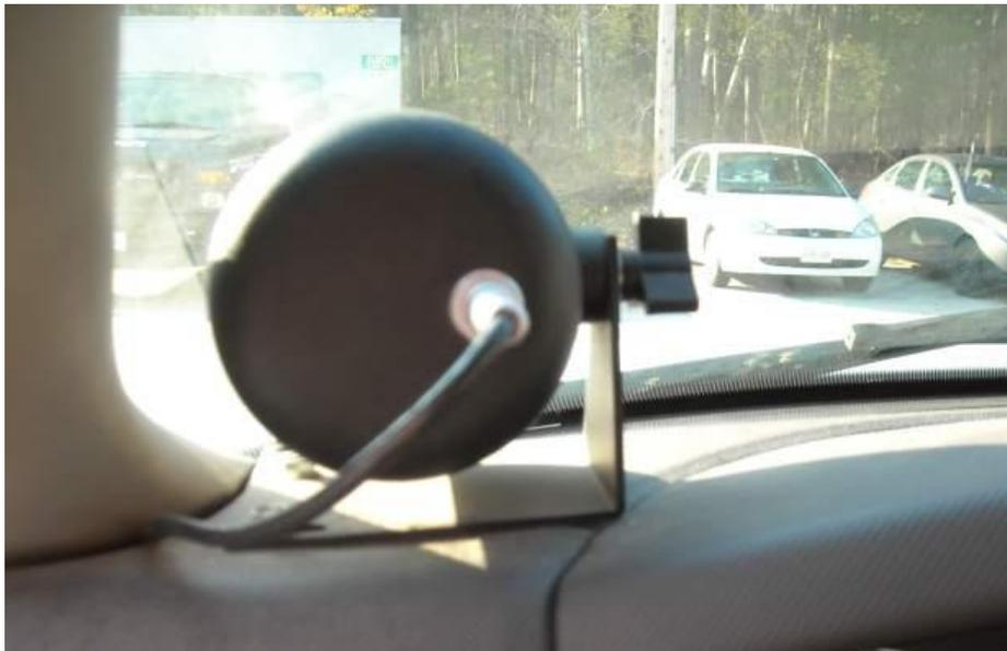
***FIGURE 12A – Front RADAR antenna bracket***
