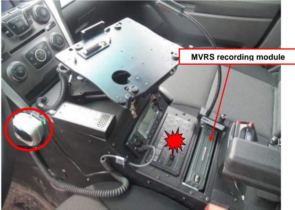
**FIGURE 18 – MVRS modular system (recording module)**
