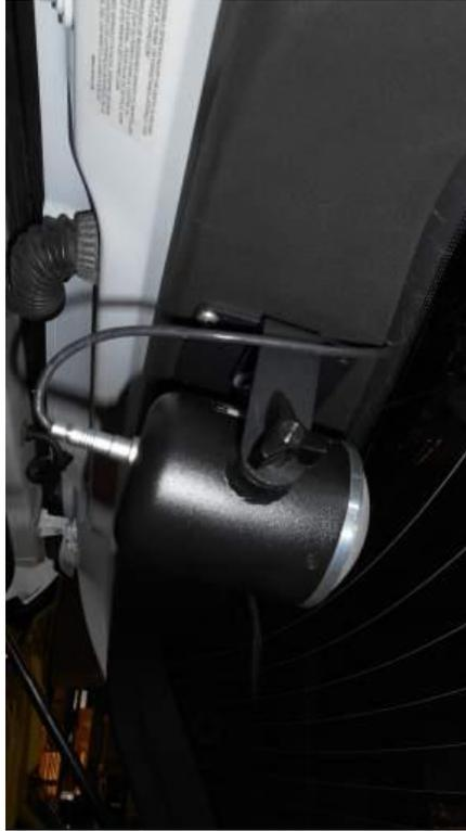
**FIGURE 12B – Rear RADAR antenna bracket**
