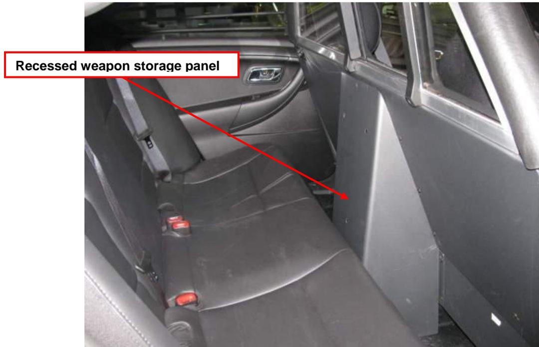
**FIGURE 20– Security screens (with recessed weapon storage panel and sliding center window)**
