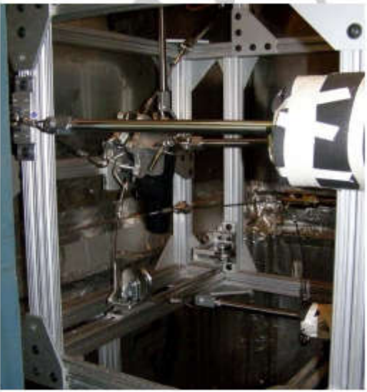
Example of Static Fixture demonstrating all directions of loading and impact testing (See Figure 1 and Figure 2)
