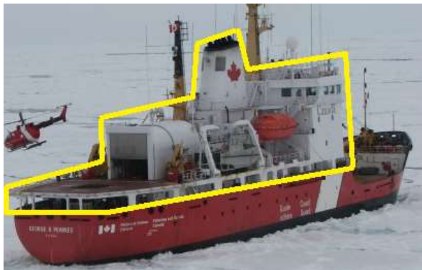
Highlight of the entire Superstructure area to have coatings renewed as part of this specification
