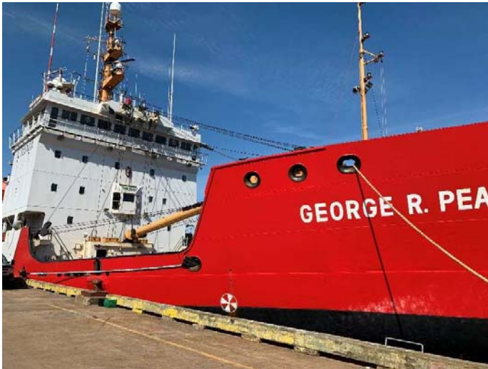
Front View – The entire superstructure, starting from the forward bulkhead of the Wire Leads Compartment on the main deck, must have the coatings renewed.
