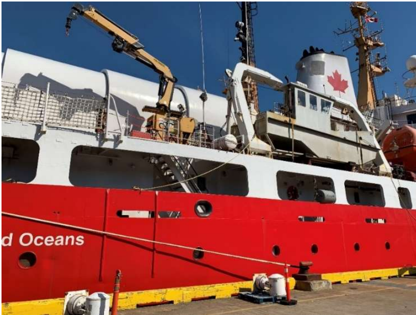
Side view of the upper deck. Both the internal and external sections (white), as well as the complete deckhead area, must be completely cleaned, prepped and coated as detailed in this specification.
