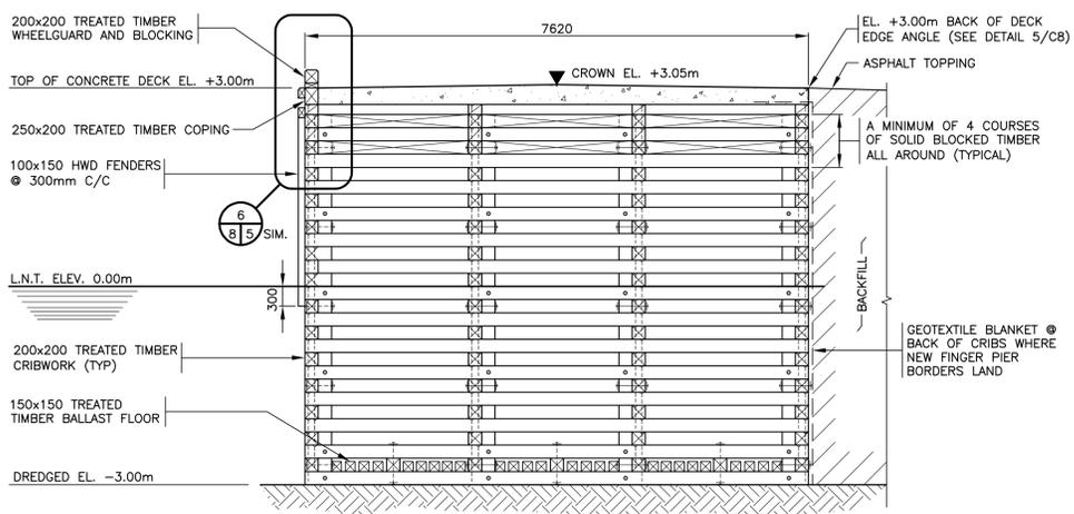
SECTION - NEW FINGER PIER WHARF (PHASE 1) SCALE: 1:50
