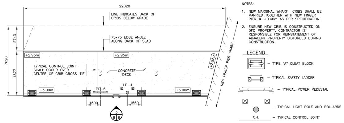
PLAN - NEW MARGINAL WHARF DECK LAYOUT (PHASE 1) SCALE: 1:100
