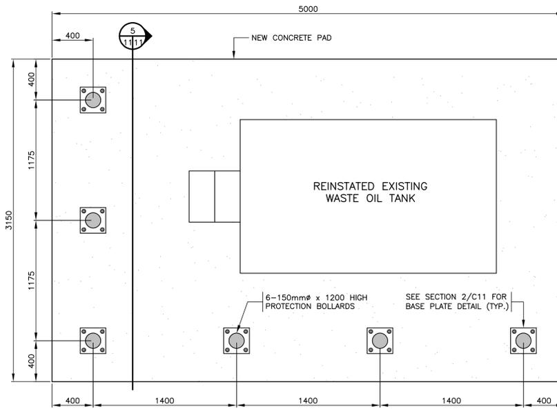
NOTE: SEE SECTION 2/C11 FOR SIMILAR BOLLARD DETAILS. THE ABOVE BOLLARDS ARE 150mm AS APPOSED TO THE SMALLER DIAMETER PROTECTION BOLLARDS FOR USE ON WHARF DECKS AT LIGHT POLES.
