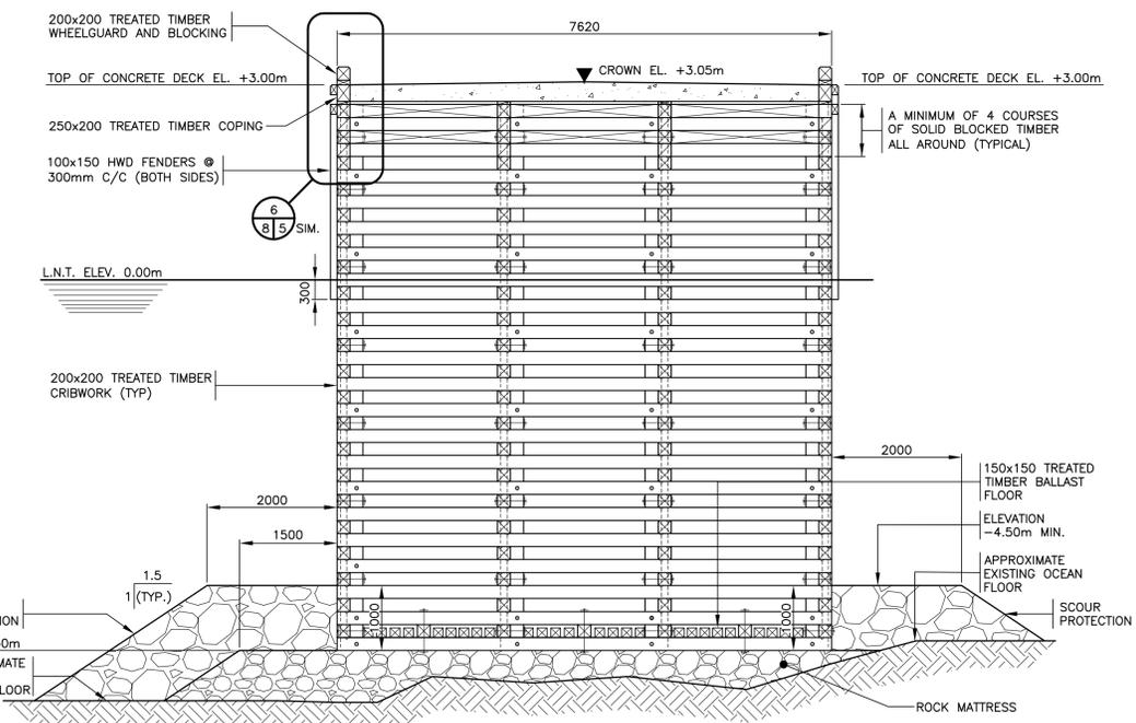
SECTION - NEW FINGER PIER WHARF (PHASE 1) SCALE: 1:50
