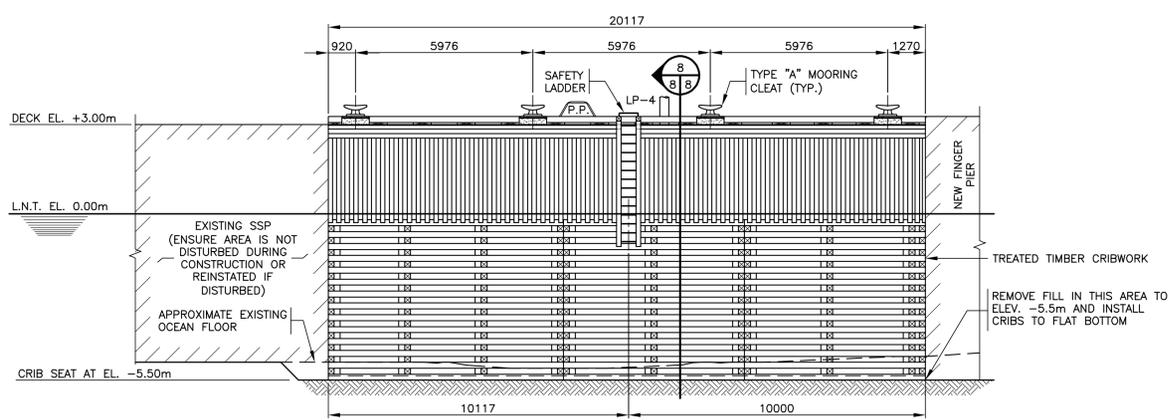
ELEVATION - NEW MARGINAL WHARF (PHASE 1) SCALE: 1:100
