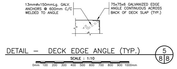
DETAIL - DECK EDGE ANGLE (TYP.) SCALE: 1:10
