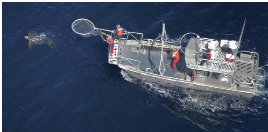
Figure 1 An example landing craft with a custom bowsprit /bow walk built over a bow gate, as well as a secondary viewing platform above the cabin used for sea turtle research (research conducted under NOAA-ESA permit #15634). Photo credit: Joel Schumacher
