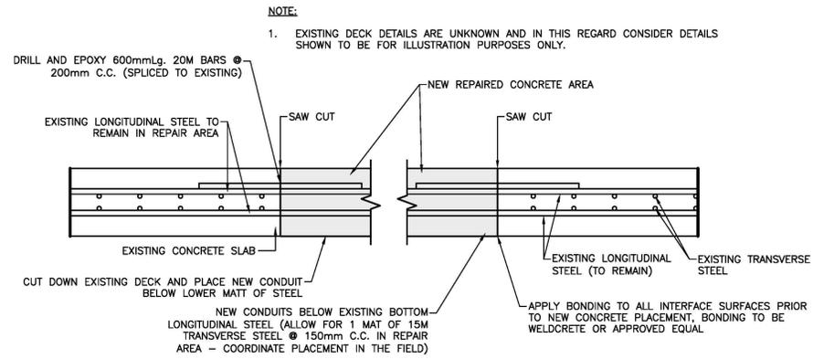
**DETAIL WHERE CONDUIT IS TO BE INSTALLED IN EXISTING WHARF DECK**
