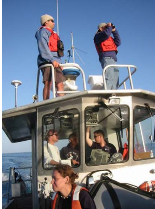
Figure 2 An example landing craft with a secondary viewing platform above the cabin roof, equipped with hand rails. Photo accessed from: https://mlml.sjsu.edu/marineops/gallery/
