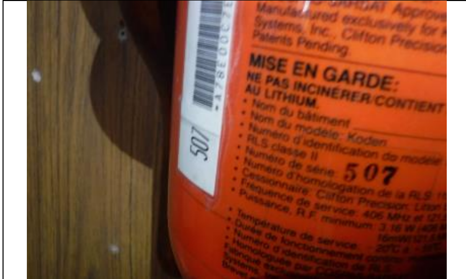
3. Lithium Batteries in EPIRB and SARTS in wheelhouse.
