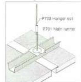
Ceiling/Partition Installation
