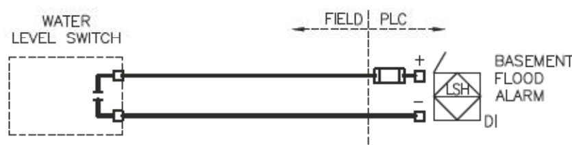
BASEMENT FLOOD SWITCH (BFS-102)
