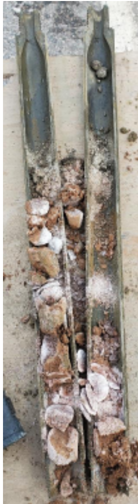
Pictures from left to right: Picture 1 - Split-spoon samples of the granular fill. Picture 2 - Boulder fill. Picture 3 - Moderately weathered alkali feldspar Granite rock core.
