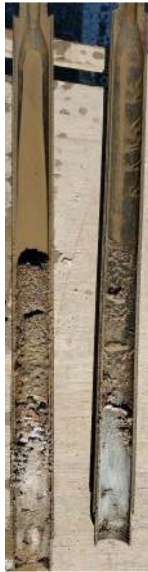
Pictures from left to right: Picture 1 & 2 - Split-spoon samples of the granular fill. Picture 3 - Granite rock core.
