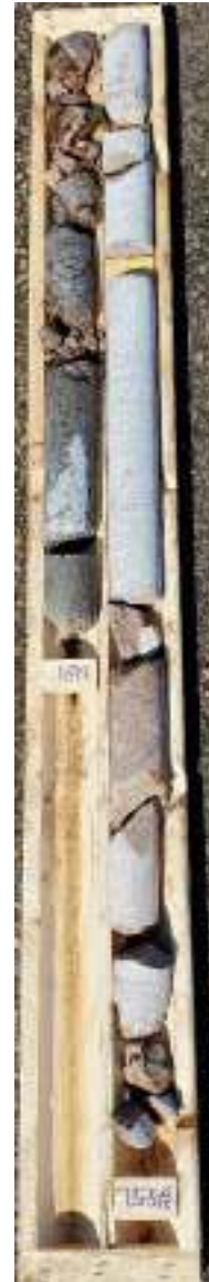
Pictures from left to right: Picture 1 & 2 - Split-spoon samples of the granular fill. Picture 3 - Granite rock core.
