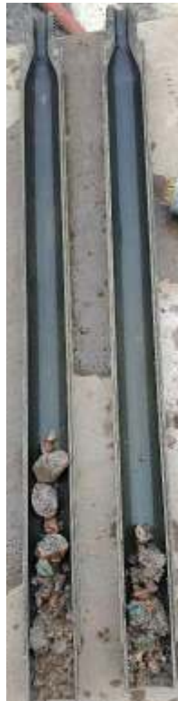
Pictures from left to right: Picture 1 - Split-spoon samples of the granular fill. Picture 2 - Boulder fill. Picture 3 - Moderately weathered alkali feldspar Granite rock core.
