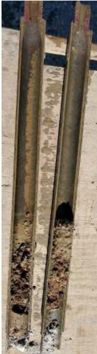
Pictures from left to right: Picture 1 & 2 - Split-spoon samples of the granular fill. Picture 3 - Granite rock core.
