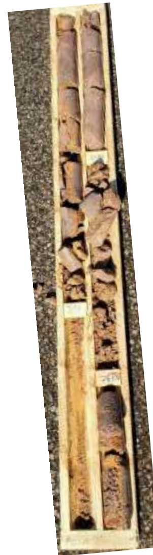
Pictures from left to right: Picture 1 - Split-spoon samples of the granular fill. Picture 2 - Boulder fill. Picture 3 - Moderately weathered alkali feldspar Granite rock core.
