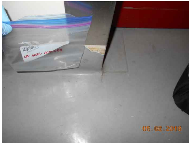
Photo 15. Sample locations LB-ADRI-ACM-08A to C; light grey vinyl sheet flooring by R.449.
