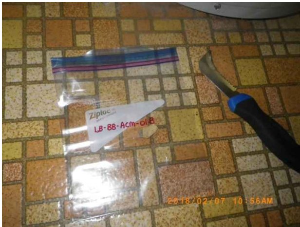
Photo 63. Sample location LB-B8-ACM-01B; yellow brick pattern vinyl flooring.
