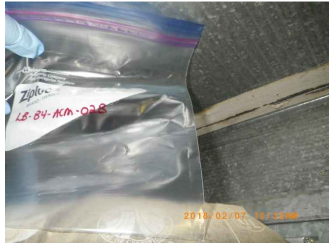
Photo 44. Sample location LB-B4-ACM-02B; paper-wrap around ducting (sample not analyzed based on confirmed asbestos in sample LB B4-ACM-02A).
