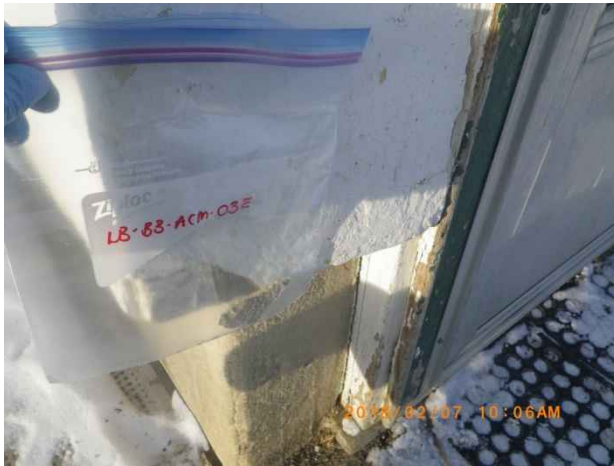
Photo 37. Sample location LB-B3-ACM-03C; exterior plaster (multi layers).
