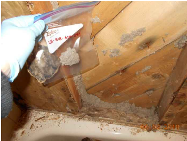
Photo 91. Sample locations LB-B18-ACM-04A to C; wall insulation from bathroom.
