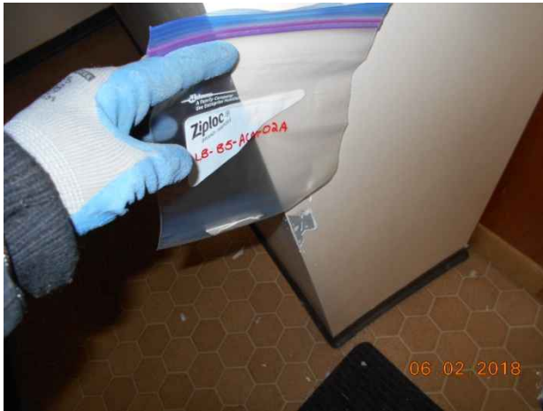
Photo 49. Sample location LB-B5-ACM-02A; dry wall/mud joint compound in front entry closet.
