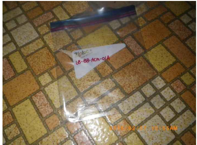
Photo 62. Sample location LB-B8-ACM-01A; yellow brick pattern vinyl flooring.
