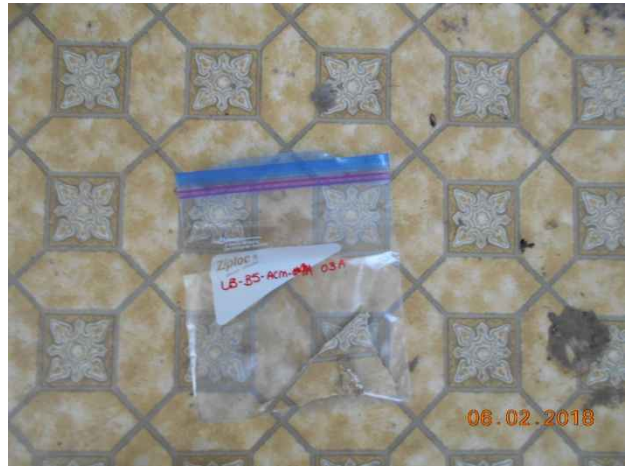
Photo 52. Sample locations LB-B5-ACM-03A to C; light yellow star patterned floor tile and backing. Confirmed asbestos-containing material (40% Chrysotile).
