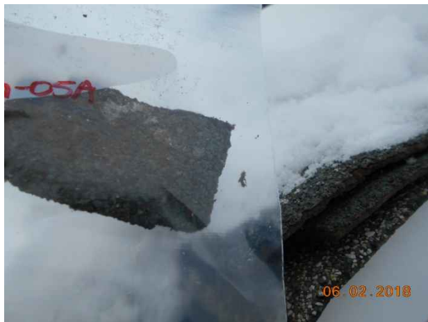
Photo 77. Sample locations LB-LB-ACM-05A to C; green roof shingles (top layer).
