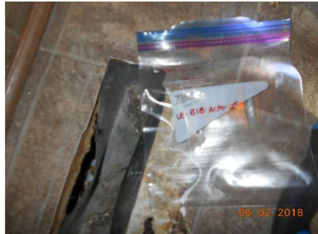
Photo 92. Sample locations LB-B18-ACM-05A to C; pebble pattern vinyl floor tile (second layer) in bathroom. Confirmed asbestos-containing material (35% Chrysotile).
