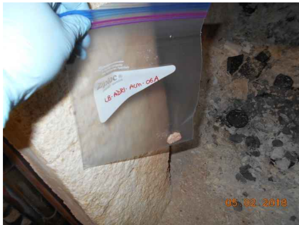
Photo 13. Sample locations LB-ADRI-ACM-06A to C; fire brick material within incinerator in R.456.
