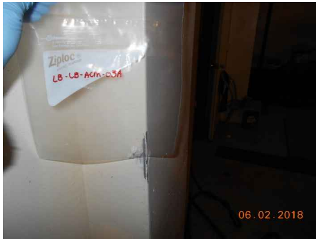
Photo 75. Sample locations LB-LB-ACM-03A to C; interior wall plaster. Confirmed asbestos-containing material (2% Chrysotile).
