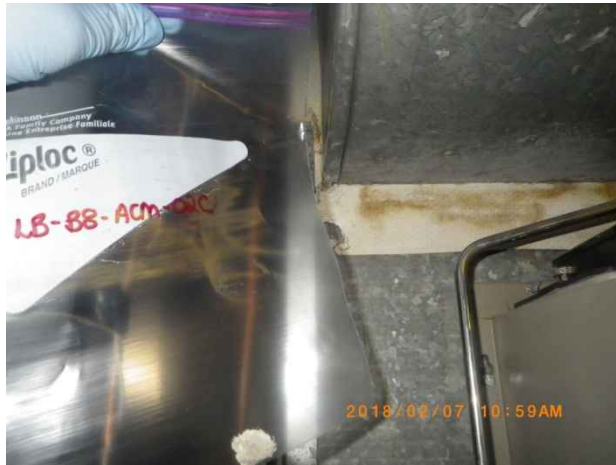
Photo 67. Sample location LB-B8-ACM-02C; paper-wrap around ducting (sampled not analyzed base on confirmed asbestos in sample LB-B8-ACM-02A).
