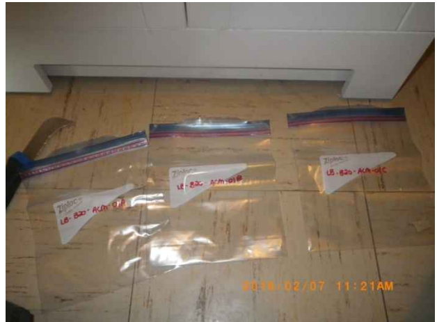
Photo 100. Sample locations LB-B20-ACM-01A to C; tan 12"x12" floor tile in basement. Confirmed asbestos-containing material (4% Chrysotile).
