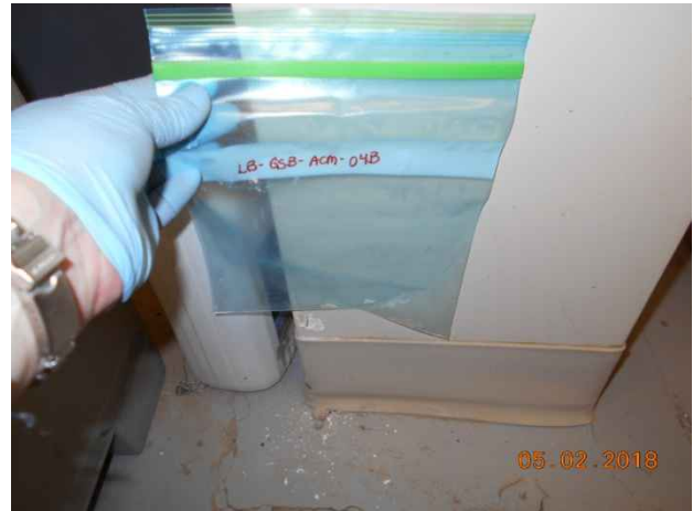
Photo 26. Sample location LB-GSB-ACM-04B; drywall mud/joint compound within the Carpenter Shop.
