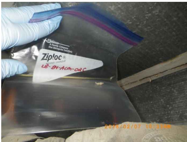
Photo 45. Sample location LB-B4-ACM-02C; paper-wrap around ducting (sample not analyzed based on confirmed asbestos in sample LB B4-ACM-02A).
