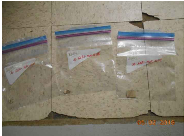
Photo 2. Sample locations LB-ADRI- ACM-01A to C; 12"12" beige/grey vinyl floor tile.
