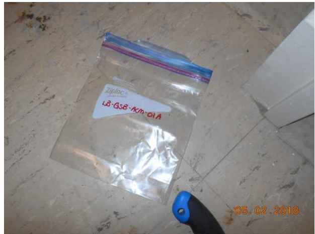
Photo 22. Samples LB-GSB-ACM-01A -C; tan 12"x12" floor tile at staircase.
