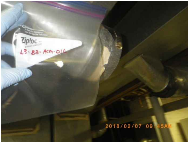
Photo 31. Sample location LB-B3-ACM-01C; paper-wrap around ducting (sample not analyzed based on confirmed asbestos in sample LB B3-ACM-01A).
