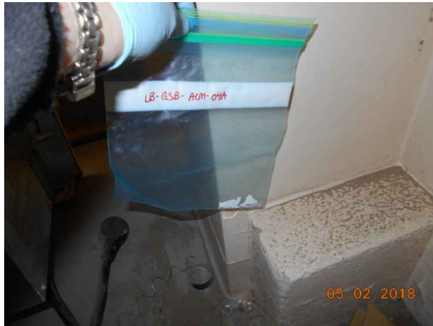
Photo 25. Sample location LB-GSB-ACM-04A; drywall mud/joint compound within Carpenter Shop.
