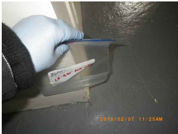
Photo 103. Sample location LB-B20-ACM-02C; drywall mud joint compound in basement bedroom closet.
