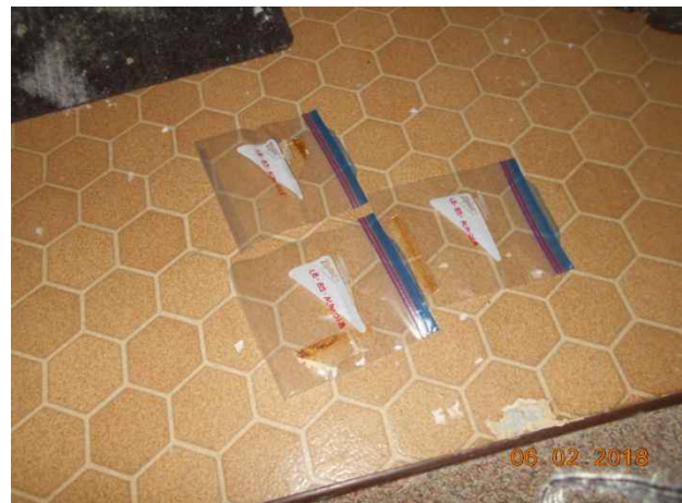
Photo 48. Sample locations LB-B5-ACM-01A to C; brown-beige hexagonal vinyl sheeting flooring.
