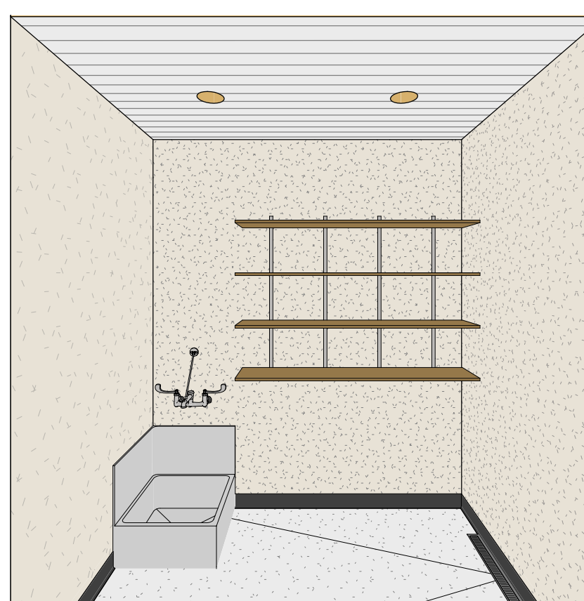
3D JANITOR ROOM - WEST WALL N.T.S.
